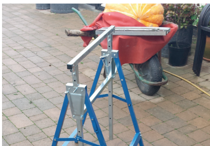
Carpenters' telescopic metal trestles are used to raise a leather sofa well above flood height.
