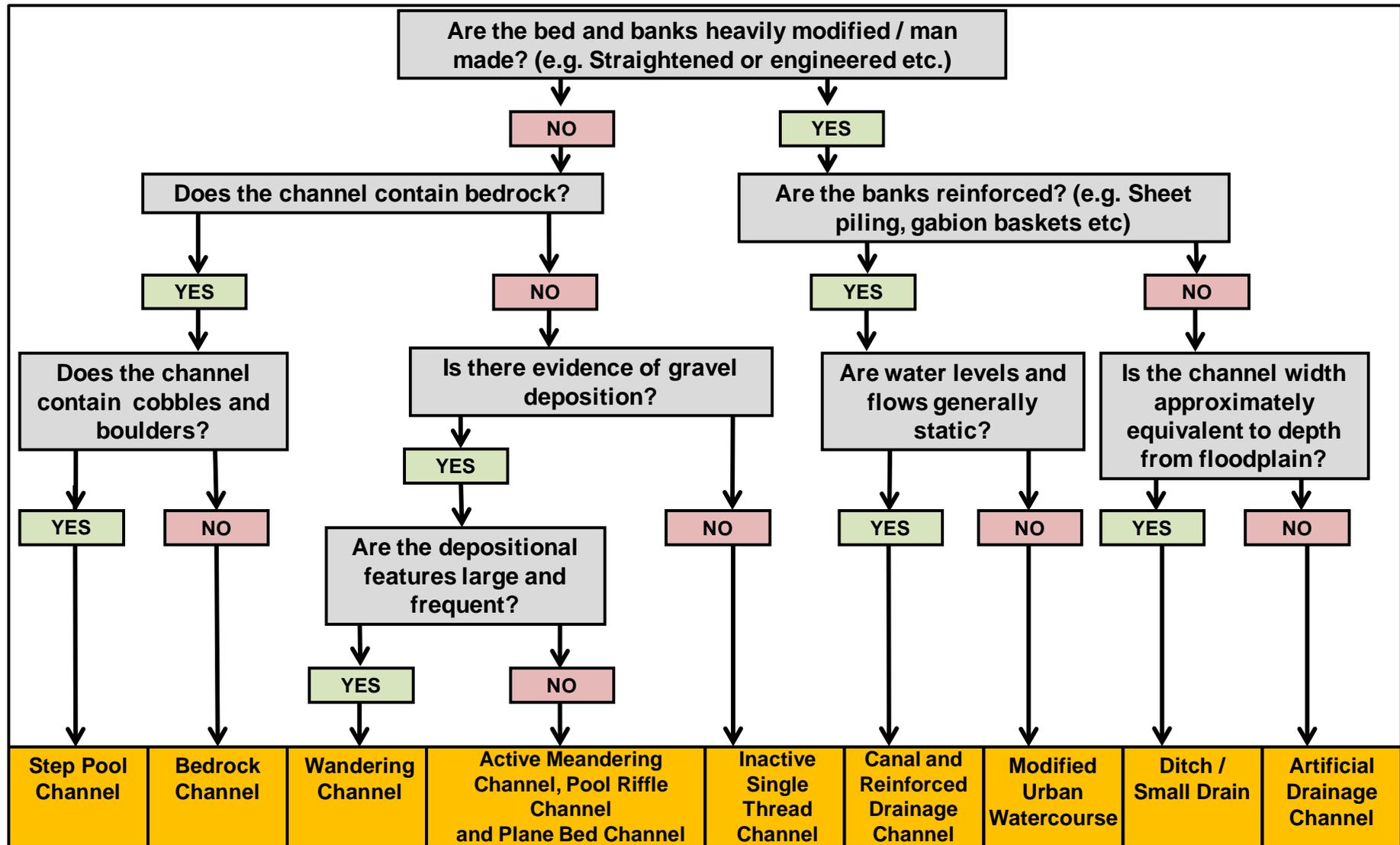
Figure 4.1 Flowchart for identifying the geomorphic watercourse type
