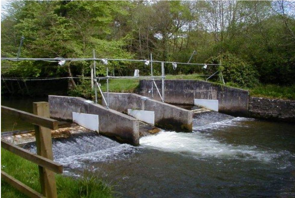
Figure 3-8 Restormel flow gauge on the River Fowey, Cornwall – a peak flow of 88 cumecs was recorded on 17 November 2010 (47 cumecs is the mean annual flood peak) – image from Environment Agency HIFLOWS website
