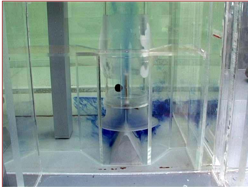
Figure 3.21: Sump model checks for pre-swirl into the pump
