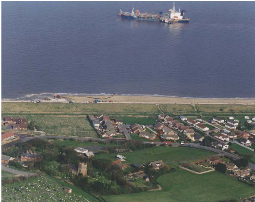
Figure 3.5 Aerial view of recharge occurring along part of the Lincolnshire coast (from CIRIA 2010)
