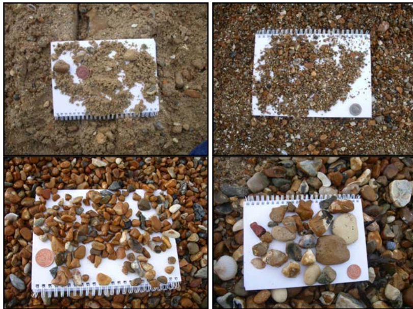
Figure 4.2 Examples of different sediment gradings (courtesy Halcrow)
