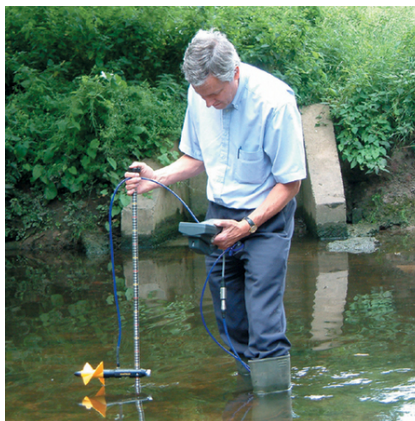
Figure A.245.1 A hand held flow meter
