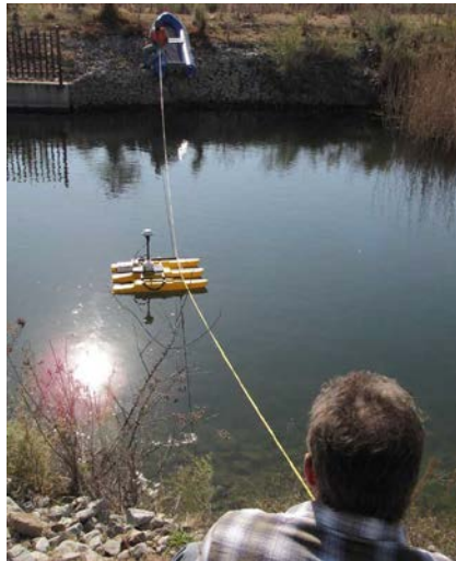
Figure A.25.2 Acoustic Doppler current profiler in use
