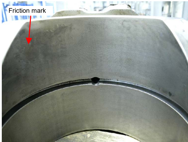
Picture 25: Connecting rod head B5; bearing surface
