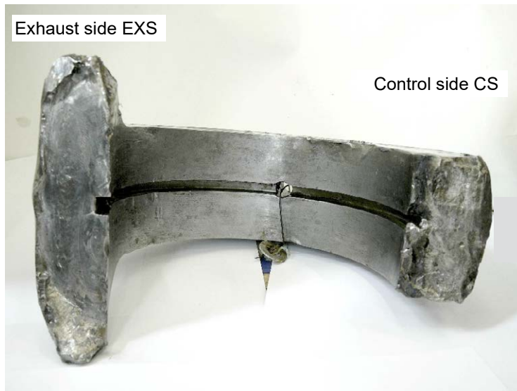
Picture 9: Connecting rod head A5; upper piece
