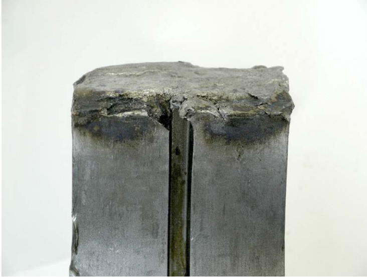
Picture 17: Connecting rod head A5; bearing surface control side (upper piece)
