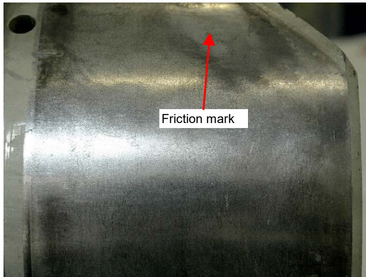
Picture 30: Bearing bush B5; backside
