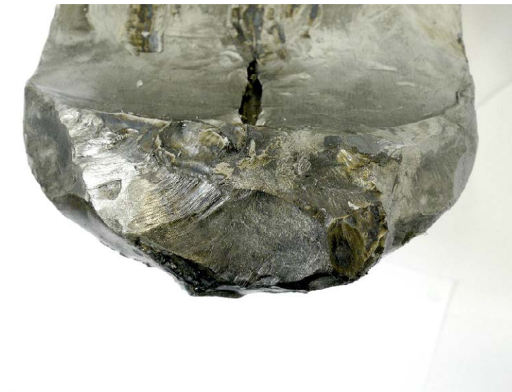
Picture 6: Connecting rod head A5; fracture surface control side
