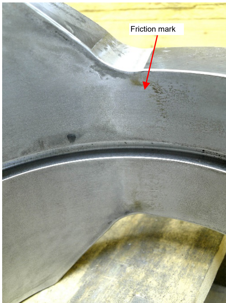
Picture 26: Connecting rod head B5; bearing surface
