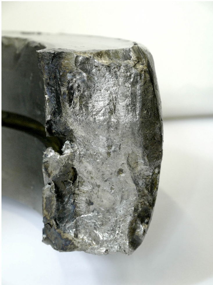
Picture 16: Connecting rod head A5; fracture surface control side (upper piece)
