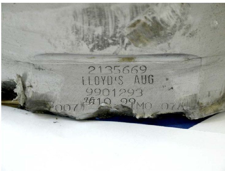
Picture 3: Connecting rod head A5; lower piece
