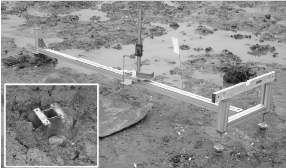
Figure 3.27 A traversing erosion beam instrument
