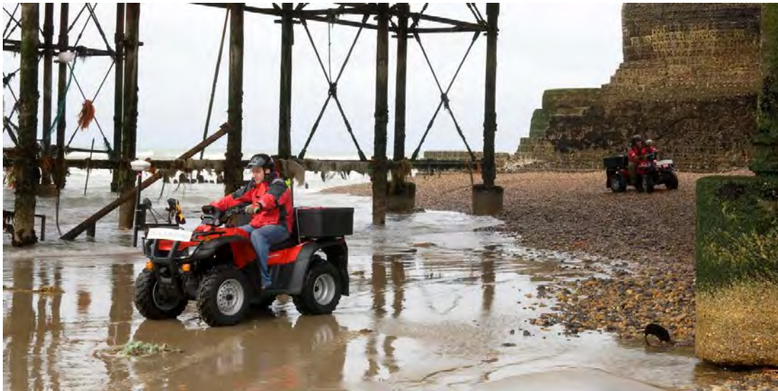
Figure 3.13 All terrain vehicle fitted with GPS equipment for coastal topographic surveying (courtesy of Worthing Borough Council)
