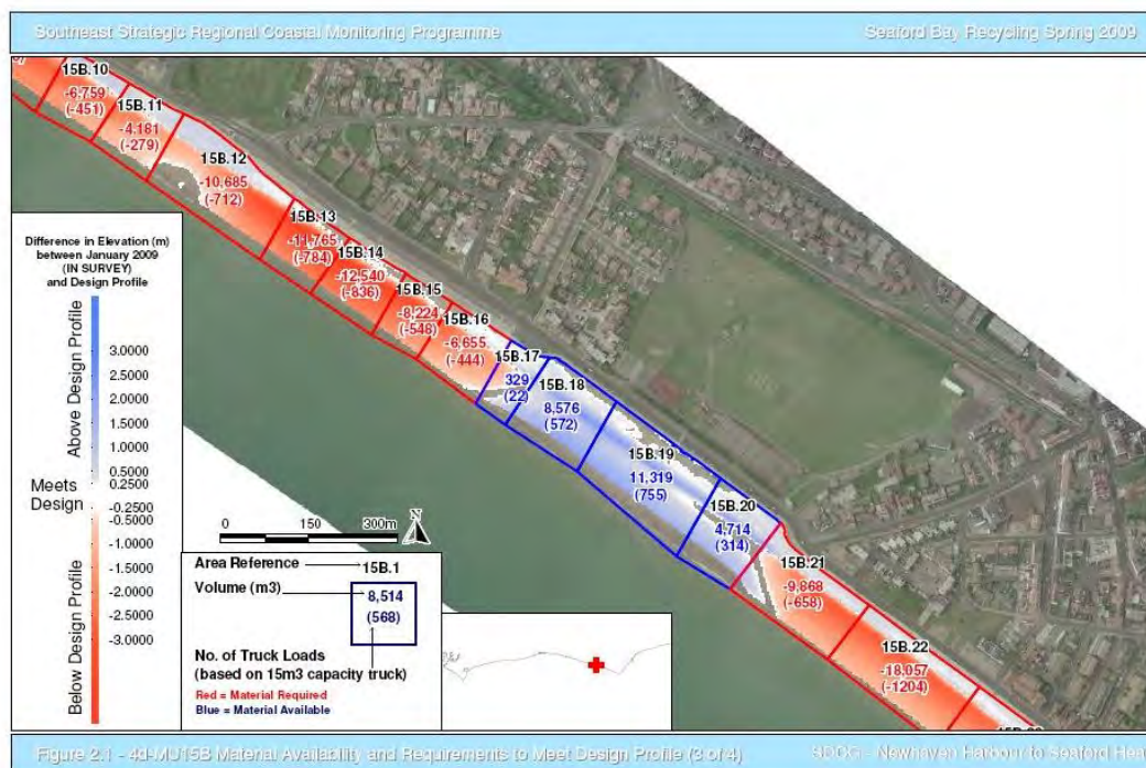
Figure 4.1 Application of monitoring data to identify beach zones beneath trigger levels (courtesy Worthing Borough Council)
