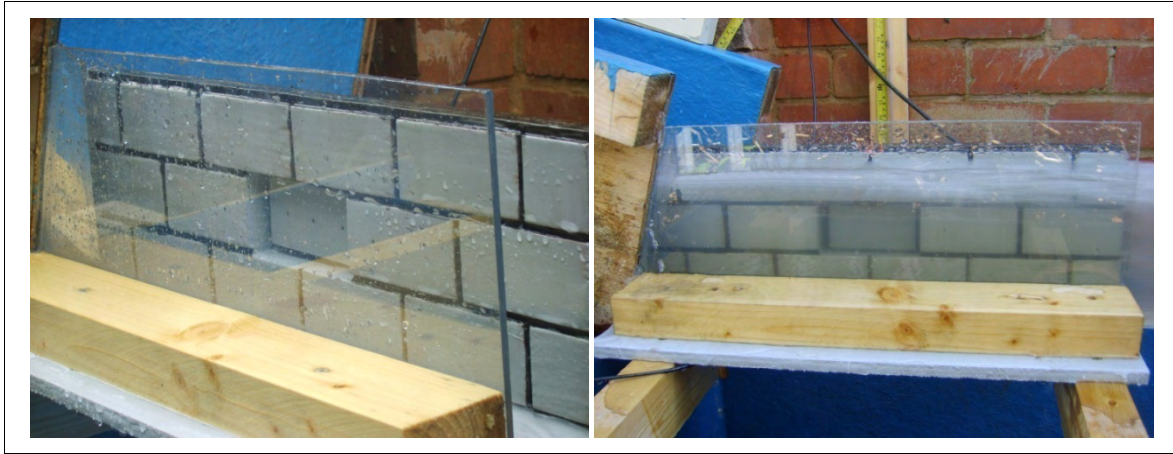
Figure 4.26 Upstream and downstream joints open - block inset by 15 mm
