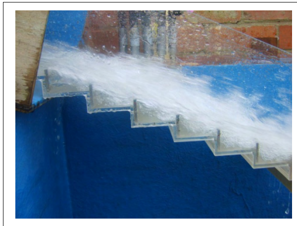
Figure 4.13 Steps with end upstands
