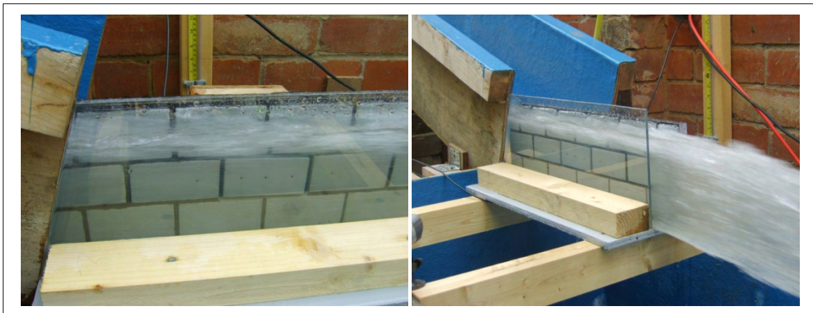
Figure 4.24 Upstream and downstream joints open - block flush
