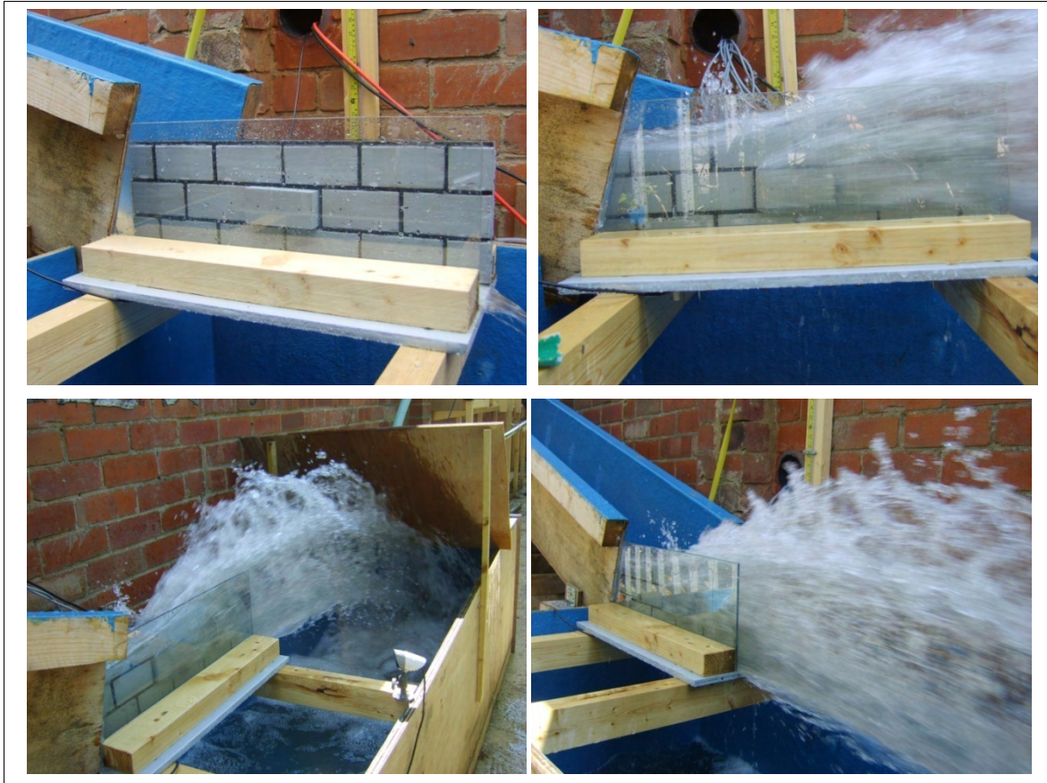
Figure 4.25 Upstream and downstream joints open - block proud by 15 mm
