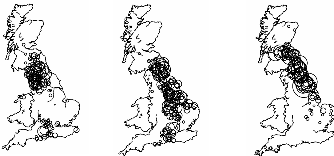
Figure 6-1: Three events, the size of the circles reflect the size of the flows at each gauging station, larger circles indicate higher flows. Only gauging stations with flows greater than QMED are shown.
