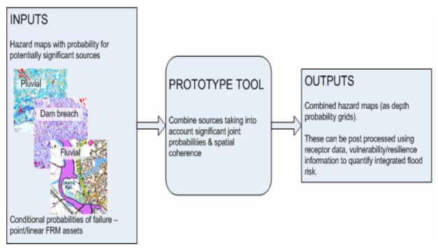
Figure 1: Schematic representation of the process of Mapping All Sources of Flood Risk.
