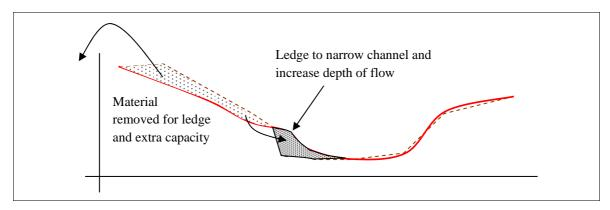
Figure 6.6 Re-profiling of a cross-section on the River Rhee
