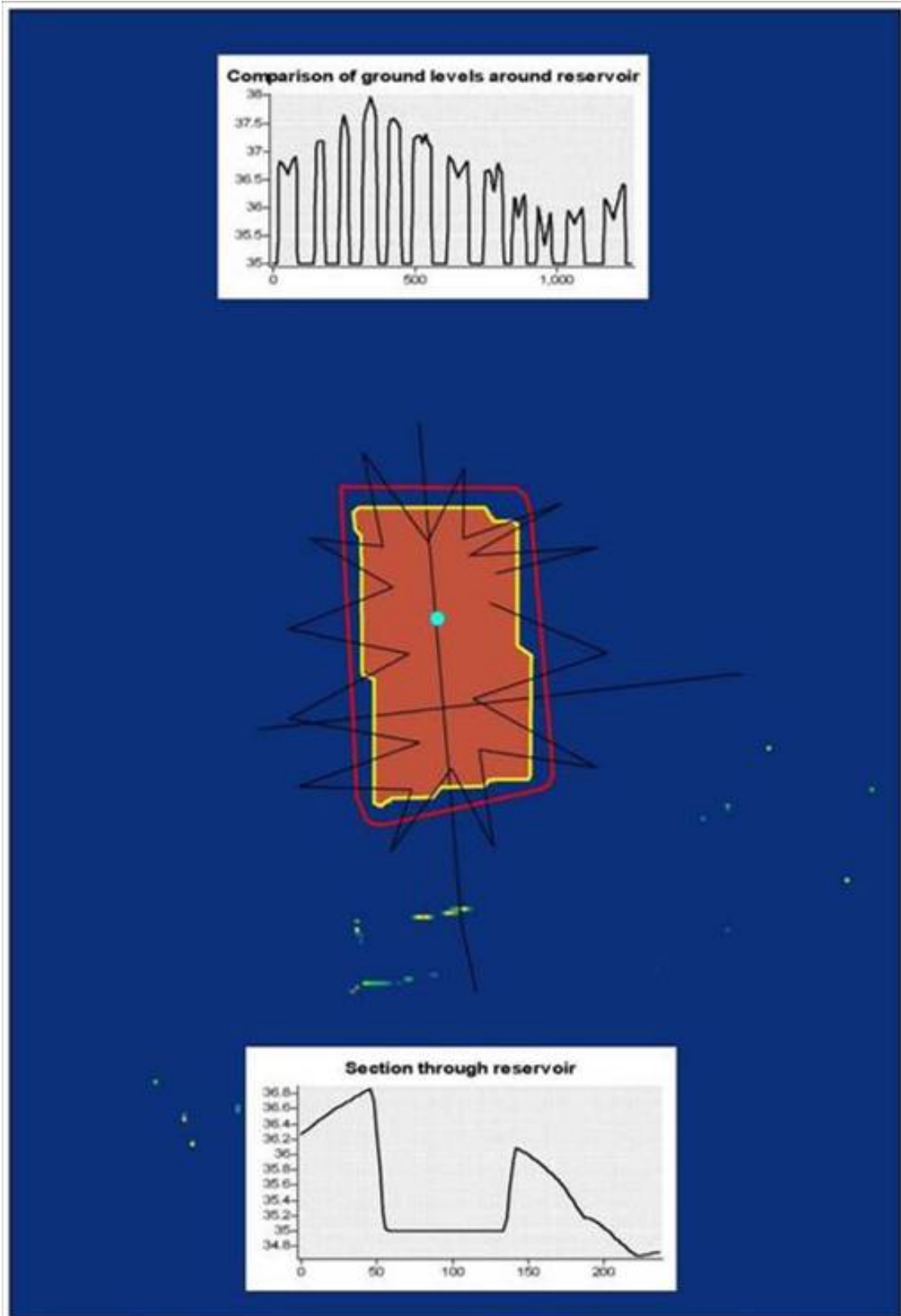
Figure D7 – View of U5007_AN in GIS software to find dam height and surface area
