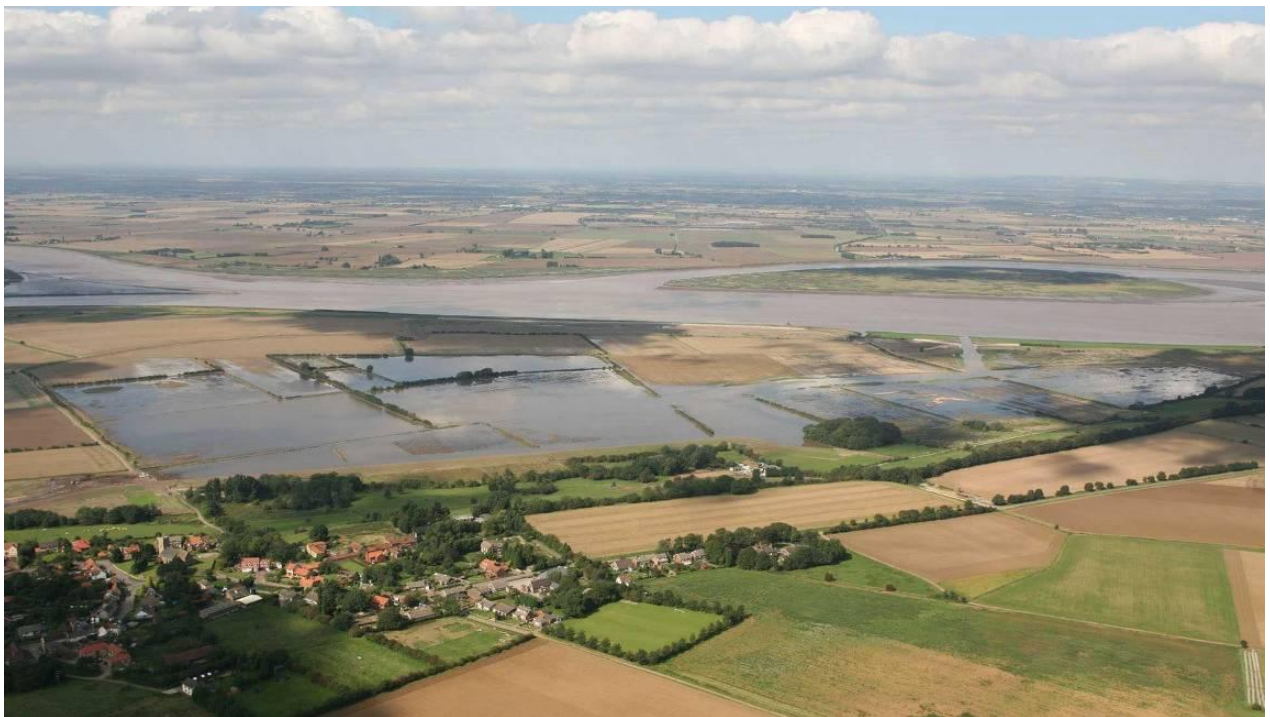
Figure 3. Alkborough Flats Managed Realignment - breach to the right. Copyright: Environment Agency
