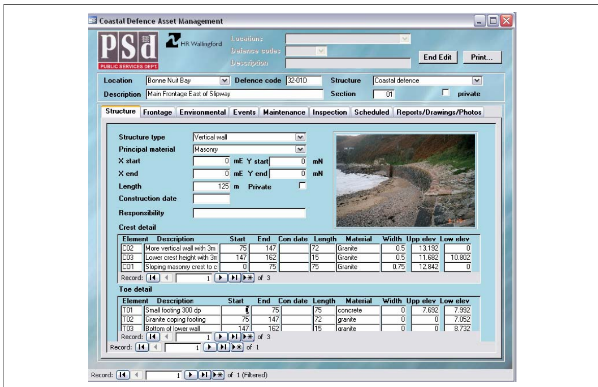
Figure 5.2 A bespoke coastal defence asset management database developed for local authority use (HR Wallingford 2002).
