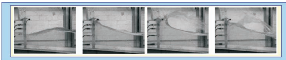
Fig. 7.18: A sequence showing the function of a parapet/wave return wall in reducing overtopping by redirecting the uprushing water seaward (back to right)
