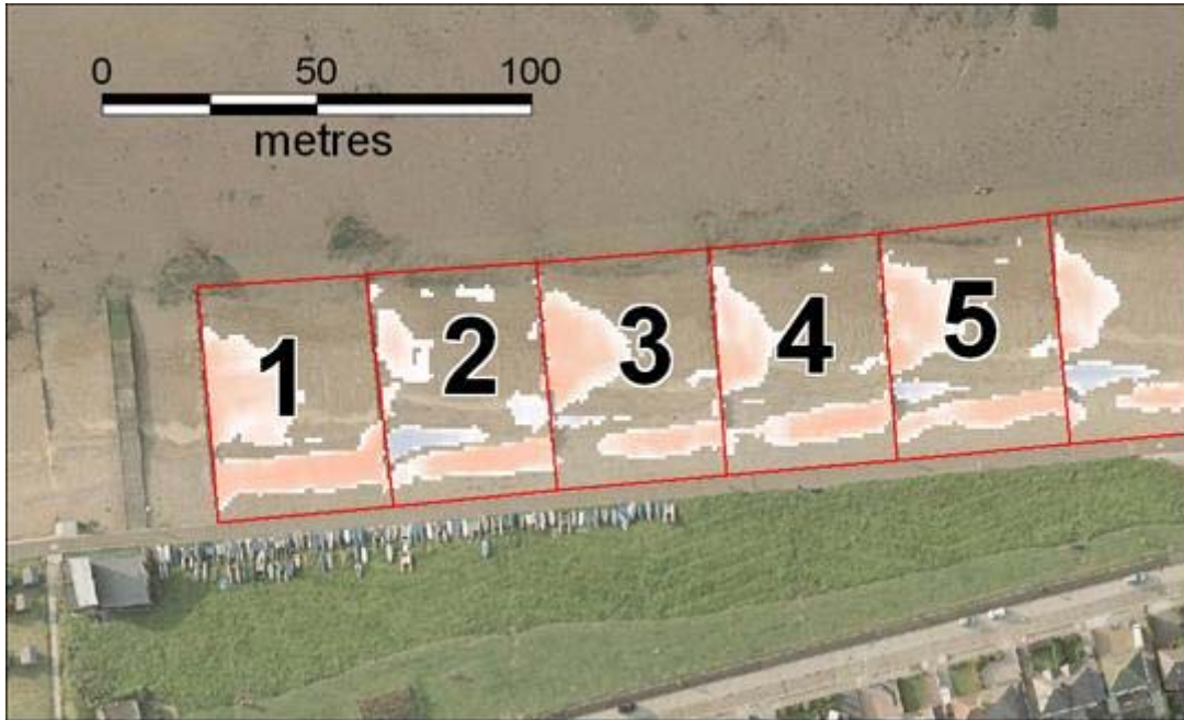
Figure 24 Map of erosion (pink-red) and accretion (pale blue-dark blue) between July 2004 and June 2007
