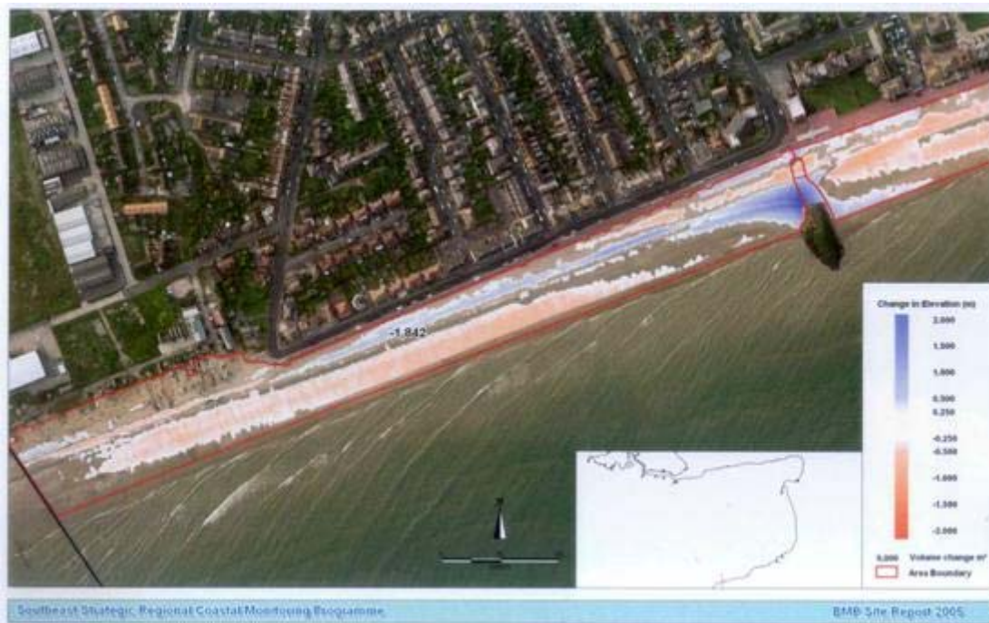
Figure 35 Volumetric analysis – a cut/fill model showing stockpile redistributed along the frontage
