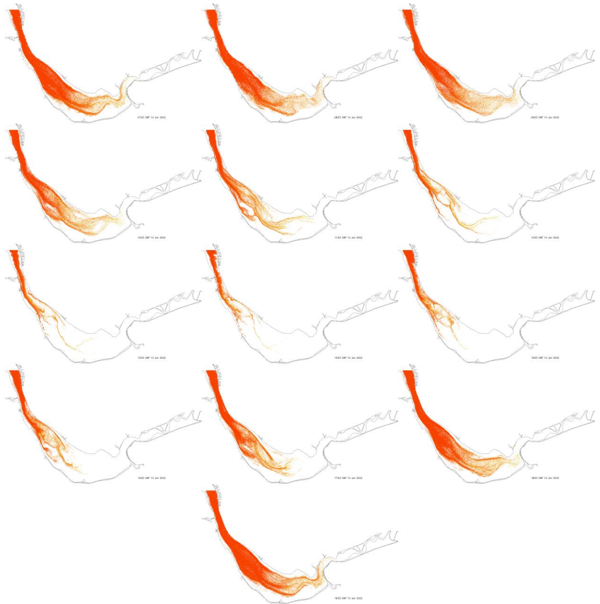
Figure 2.2 Modelled suspended tracked particles at hourly intervals in the Mersey
