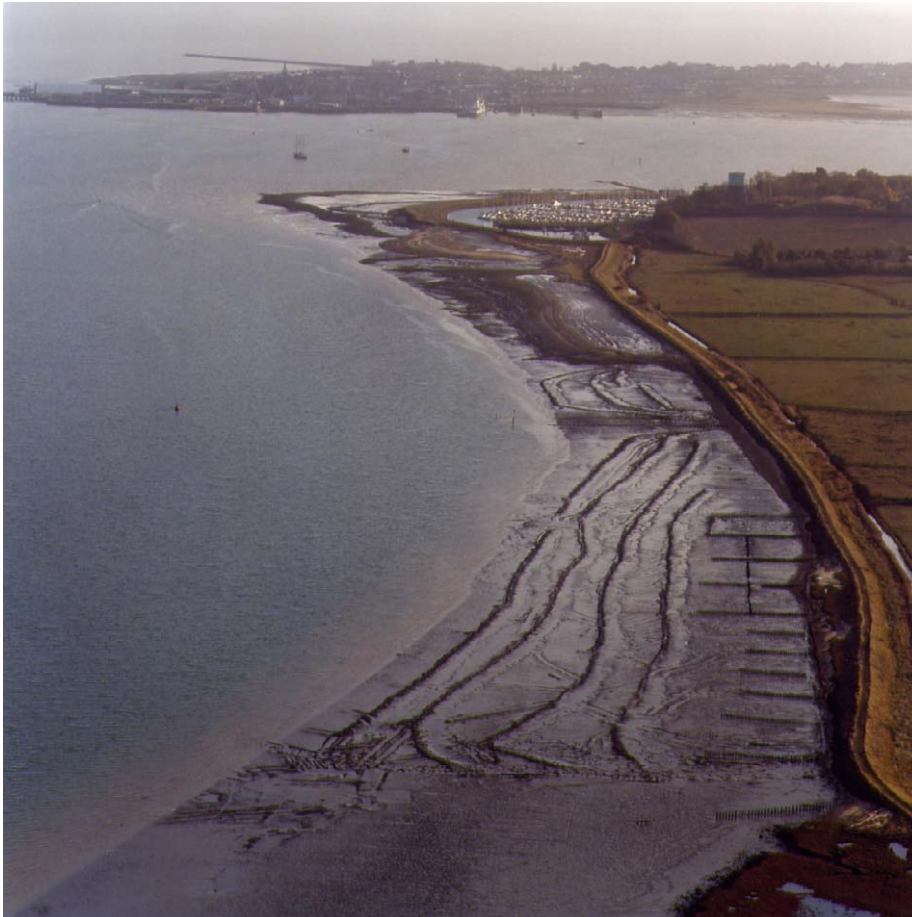
Figure 11 Photograph of bunds used to alleviate flood risk and enhance habitat
