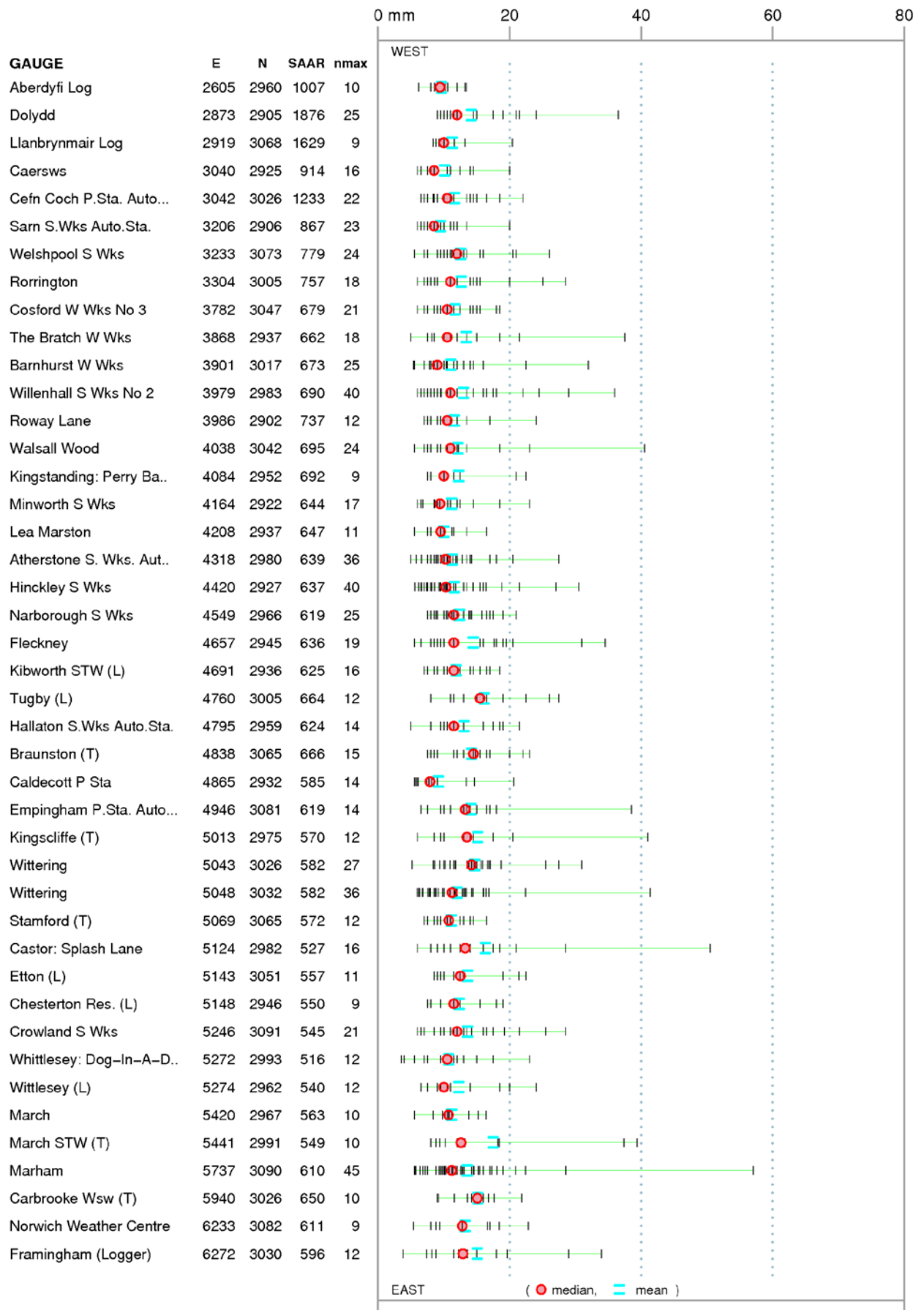
Figure A.10 1 hour annual maxima for GB raingauges between 2900 N and 3099 N
