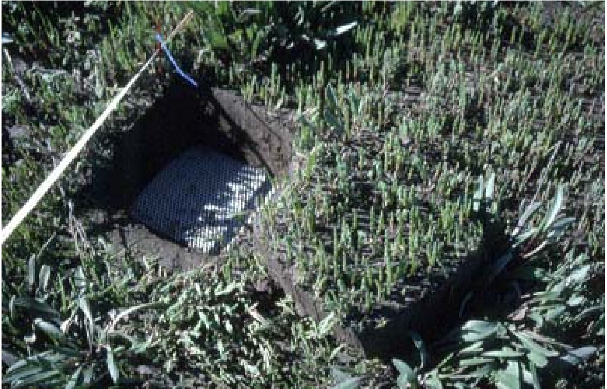
Photo 3.1. Inserting an expanded metal 'accretion' plate. Five plates were set out at random intervals along a 5m strip at each sampling site.
