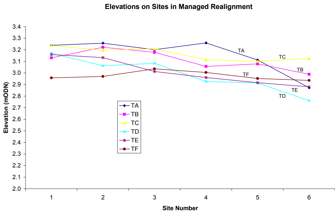
(b) Inside MR. Elevations range between 2.76 to 3.26
