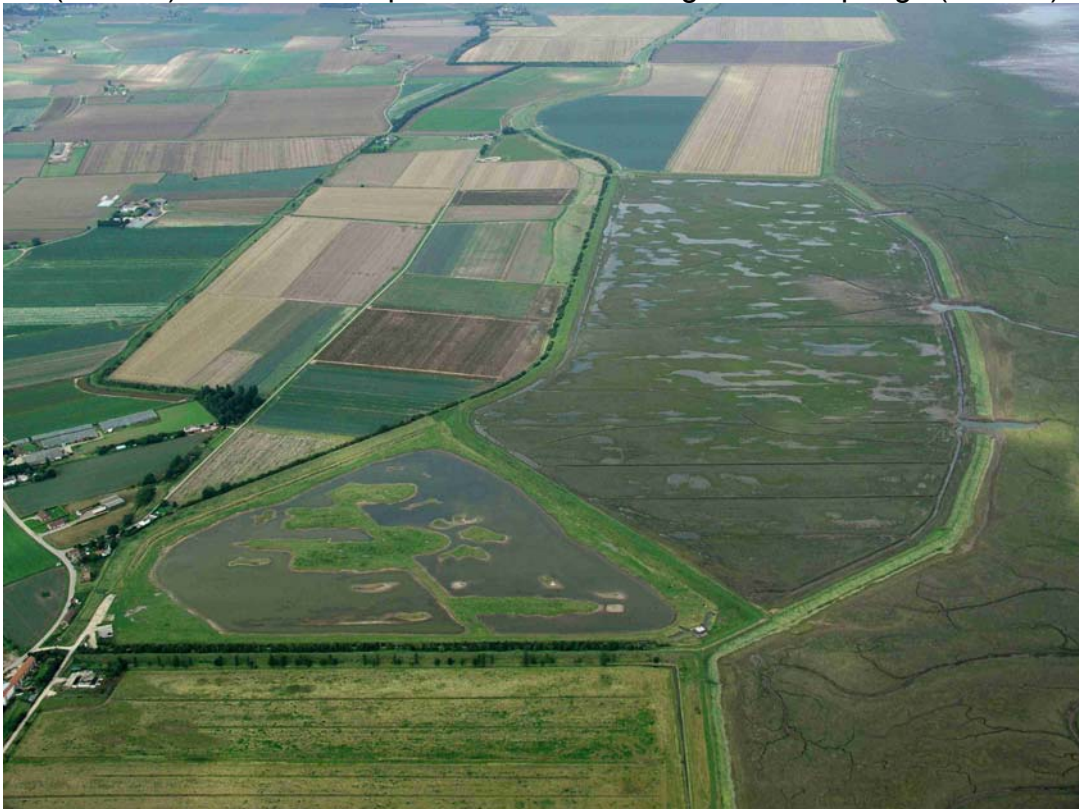
Photo 9.1. Freiston realignment site, viewed from the southern end. Note the sparsely vegetated area inside the site opposite the central breach. Photo: Environment Agency
