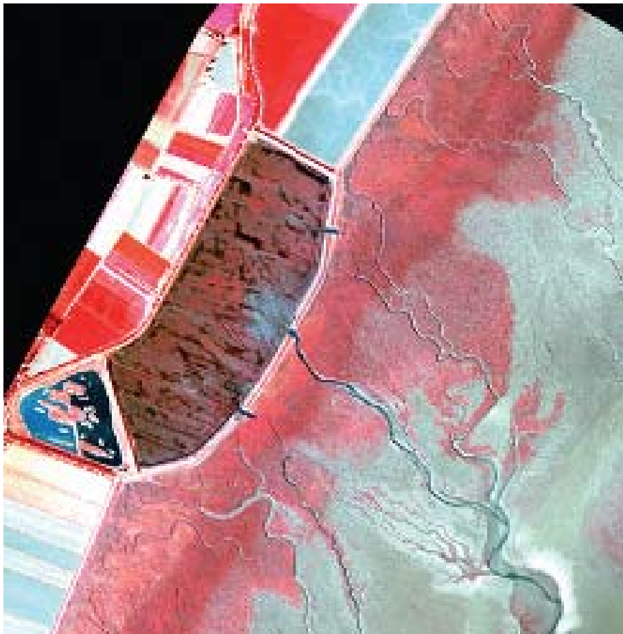
Image 3.1. Airborne Thematic Mapper Image (NERC) of Freiston Realignment and coastal salt marsh and mudflat (taken September 2003). Note the large fan-shaped area of bare sediment (blue colour) opposite the middle breach inside the site. It is also interesting to see the remnant pre-reclamation salt marsh dendritic creek patterns in the field north of the realignment site.
