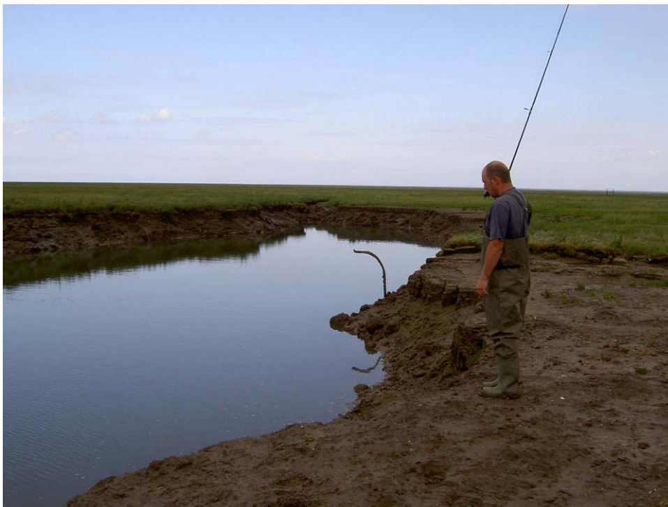
Image 7.8: Plumbing the depth of the south breach at low tide. At the time this photograph was taken, the water depth was 7 metres, too deep to sample effectively using current sampling methods.
