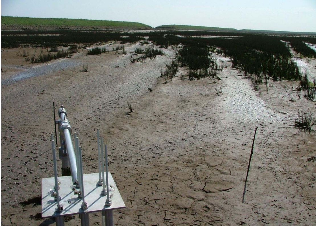
Plate 4.2. SET instrument deployed at site 7 (category: inside the managed realignment, close to the breaches; see Figure 1 for exact location), April 2005. Note less consolidated sediments infilling unvegetated former runnels at this site (photograph: S. Boreham).
