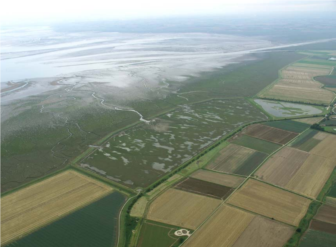
Photo 9.2. Freiston realignment site viewed from the north end. Note marked widening of the creek from the central breach, through the fronting salt marsh Photo: Environment Agency
