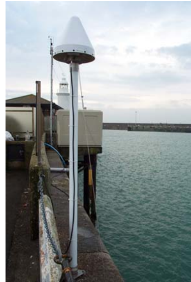
Figure 1 Photograph of a GPS antenna and monument: the photograph shows the equipment installed at the Dover tide gauge.
