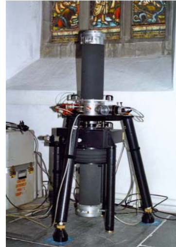
Figure 4 Photograph of the FG5 absolute gravity instrument: the photograph shows the equipment in use at the AG station near the Newlyn tide gauge.
