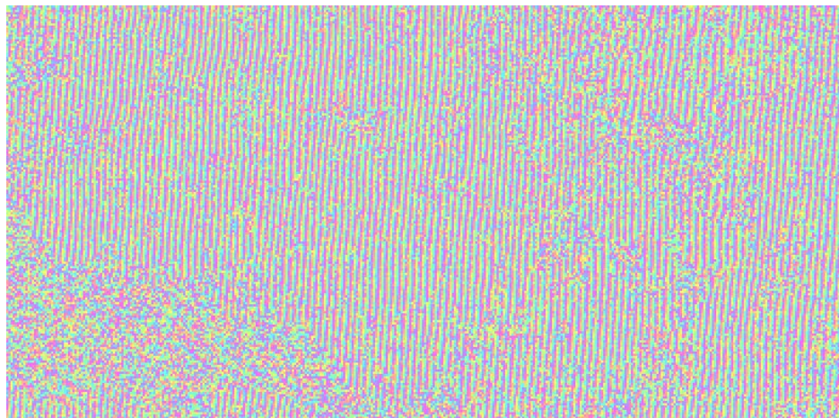
Figure 2.12 An example InSAR interferogram: reproduced from Warren (2007)
