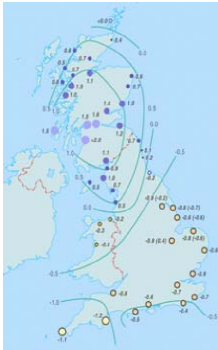
Figure 3.2 Map of estimates of changes in land level for Great Britain based on geological studies (Shennan and Horton 2002)
