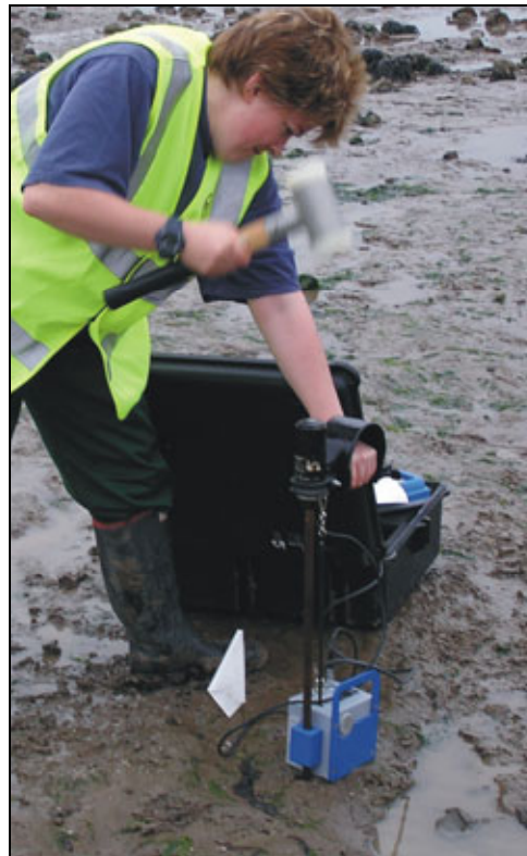
Figure 3.26. Panda penetrometer test
