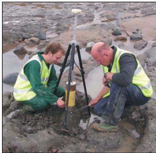
Figure 3.24. Preparation of U100 tube (triaxial) sample
