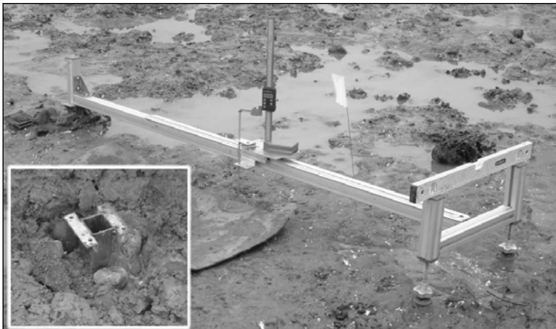
Figure 3.9. The Traversing Erosion Beam in use at Warden Point.
