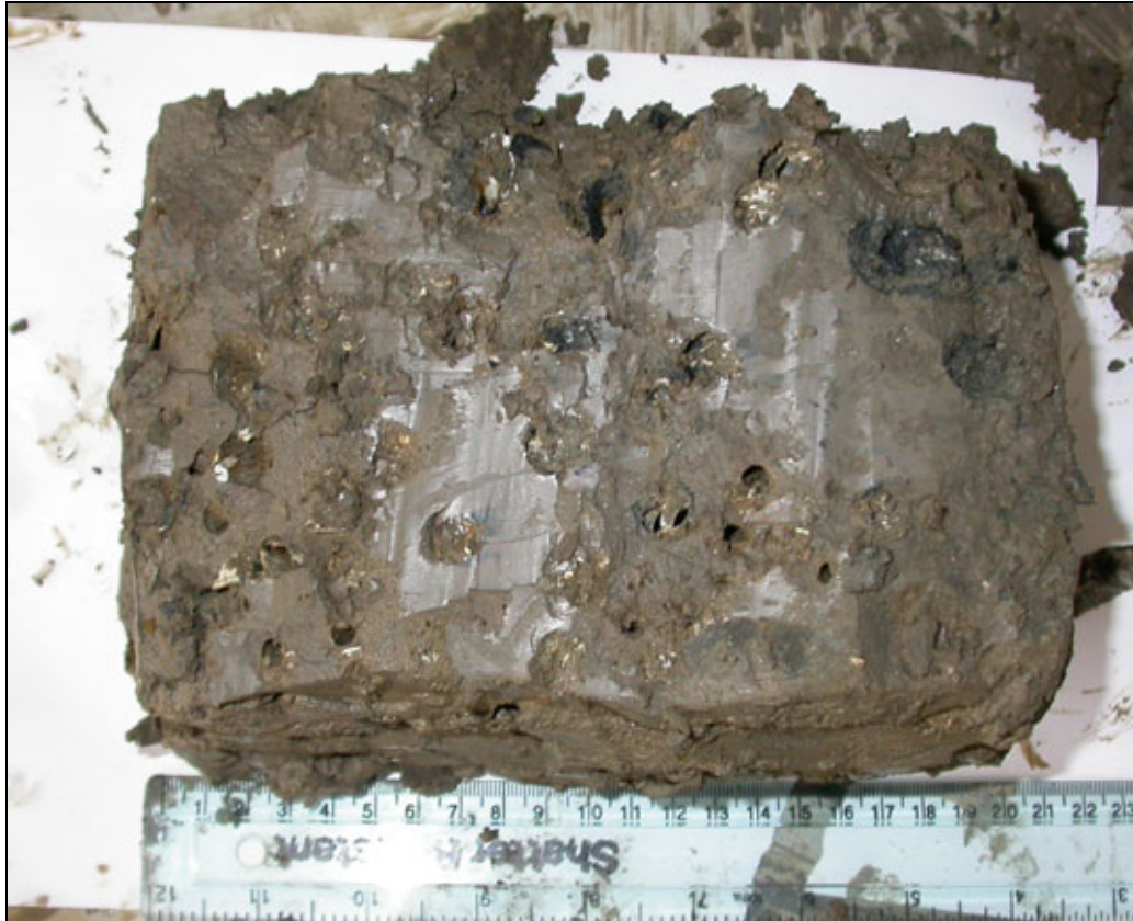
Figure 3.15. Dissected block of cohesive shore platform used to estimate piddock and borehole density.
