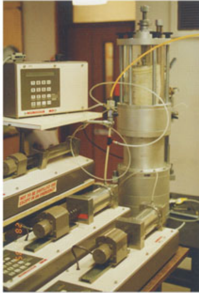
Figure 3.30. GDS (Bishop & Wesley type) 100 mm automated stress-path triaxial system.
