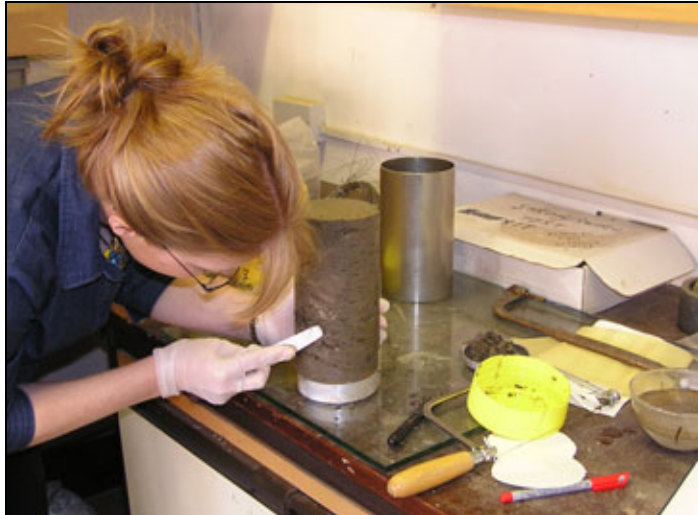
Figure 3.29. Making repairs to the triaxial test specimen.
