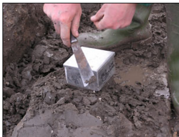
Figure 3.25. Preparation of shear-box sample
