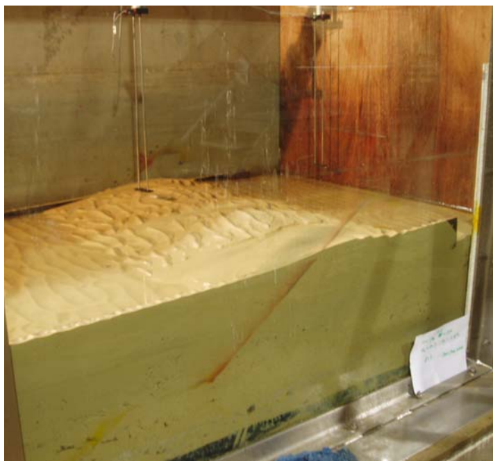
Figure 4 An example of the scour pattern at the wall after 3000 waves
