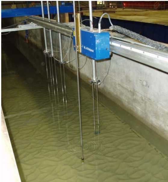
Figure 2 Bed profiler and wave gauges on the profiling rail.
