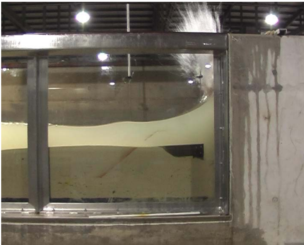
Figure 9 An example of a wave breaking directly onto the structure during test 04.
