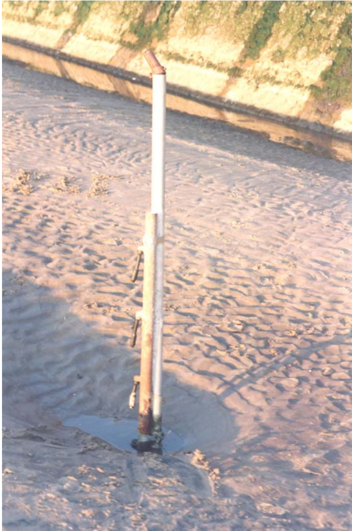
Plate 4 Offshore scour monitor installed at Blackpool
