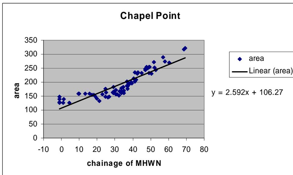
Figure 35 Cross-sectional area against chainage of MHWN for Chapel Point
