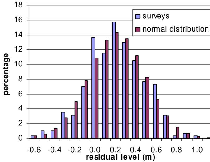
Figure 25 Measured and Gaussian distribution of residual beach levels at Boygrift Outfall
