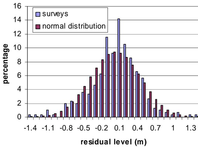
Figure 22 Measured and Gaussian distribution of residual beach levels at Trusthorpe Outfall
