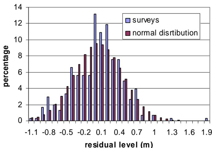
Figure 28 Measured and Gaussian distribution of residual beach levels at Jackson’s Corner
