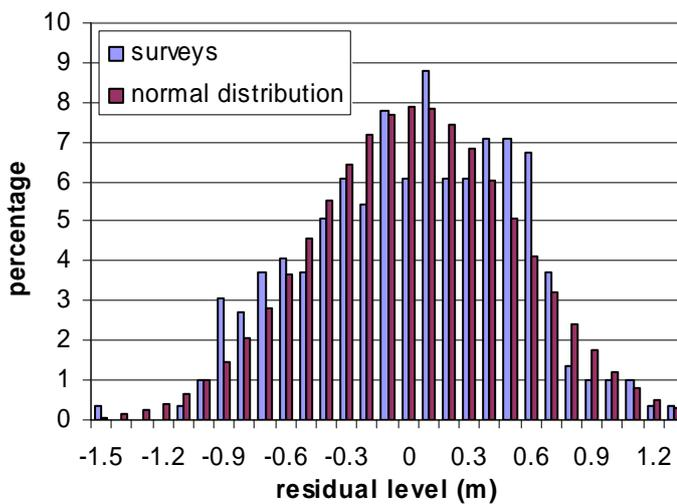
Figure 27 Measured and Gaussian distribution of residual beach levels at Trunch Lane
