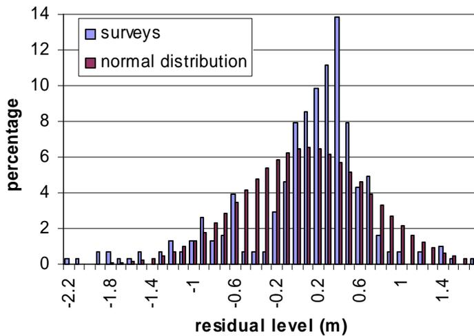
Figure 26 Measured and Gaussian distribution of residual beach levels at Chapel Point
