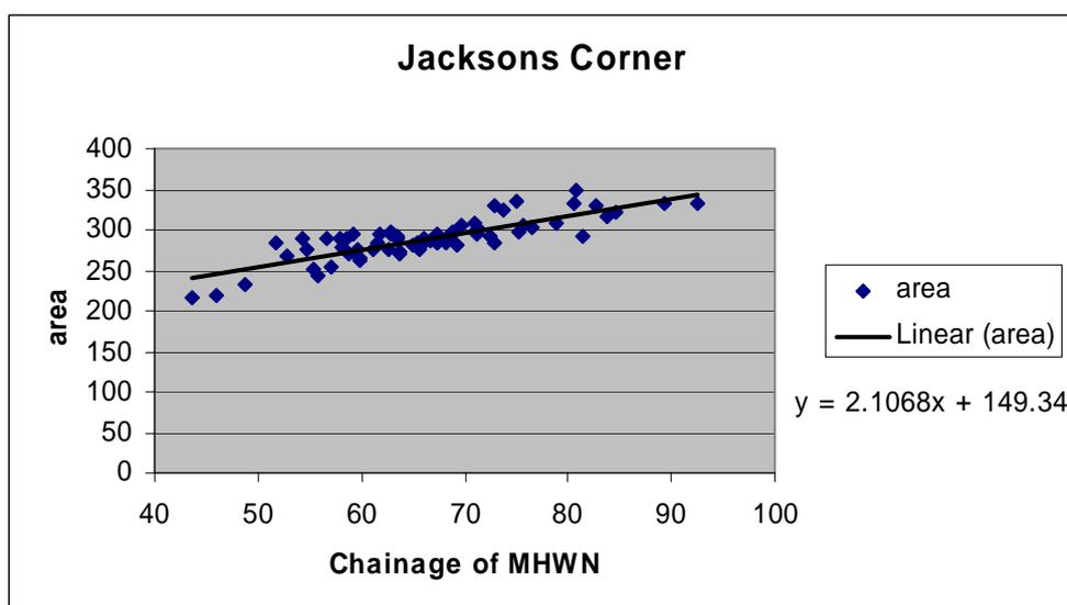
Figure 36 Cross-sectional area against chainage of MHWN for Jacksons Corner
