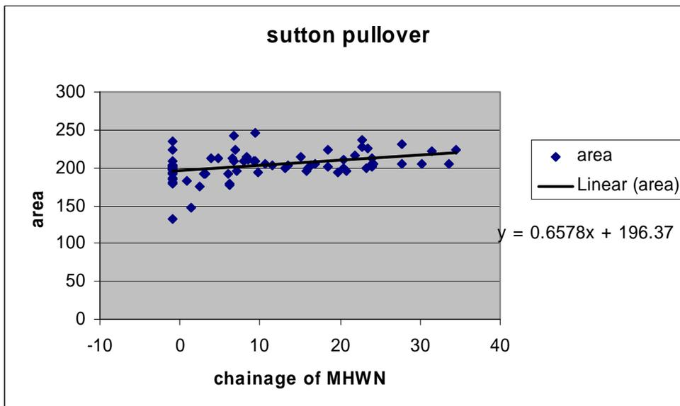
Figure 34 Cross-sectional area against chainage of MHWN for Sutton Pullover
