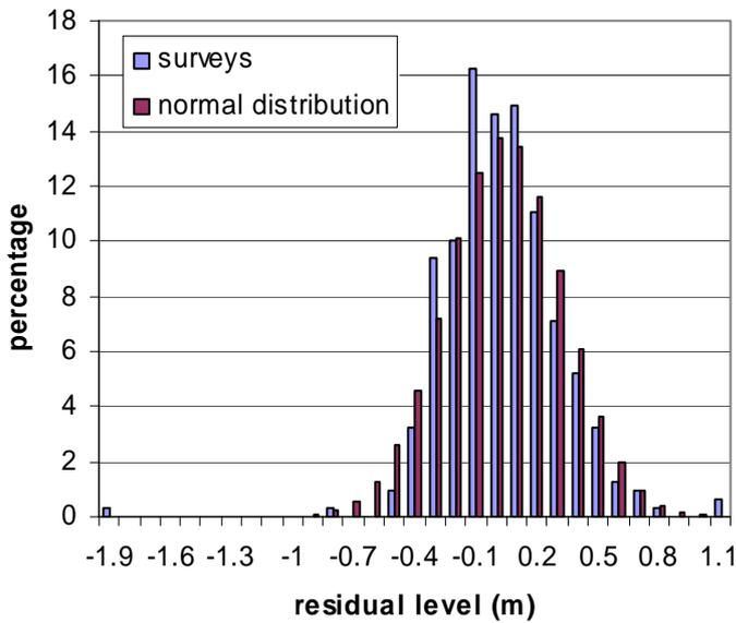
Figure 24 Measured and Gaussian distribution of residual beach levels at Sutton Pullover
