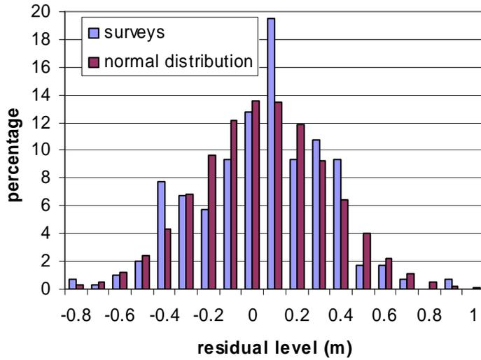
Figure 23 Measured and Gaussian distribution of residual beach levels at Bohemia Point
