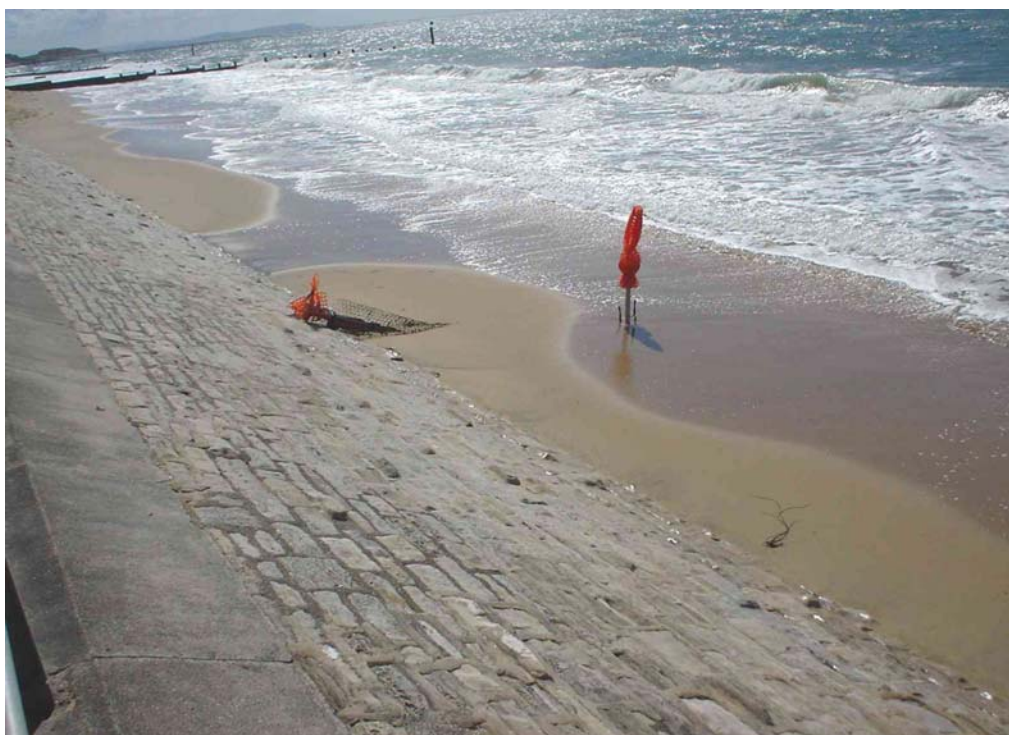
Plate 25 Scour monitors photographed near high tide on 23 May 2005.
