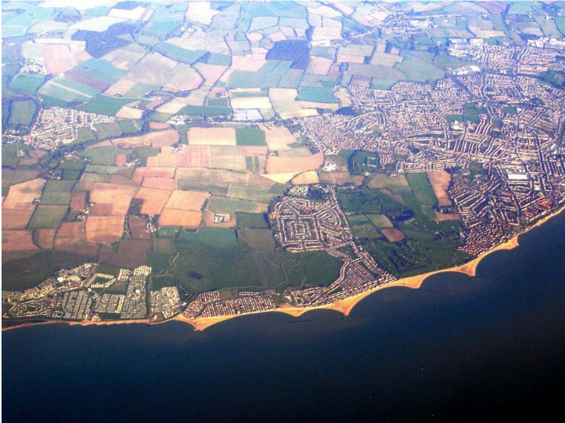
Figure 5.4 Variations in beach width caused by rock groynes at Jaywick, 2006
