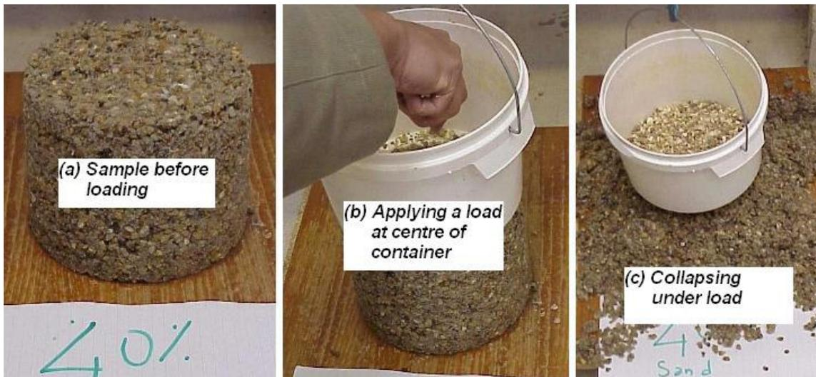
**Figure 3.9** Different stages of “sand castle” test ( $\lambda=40\%$ )
