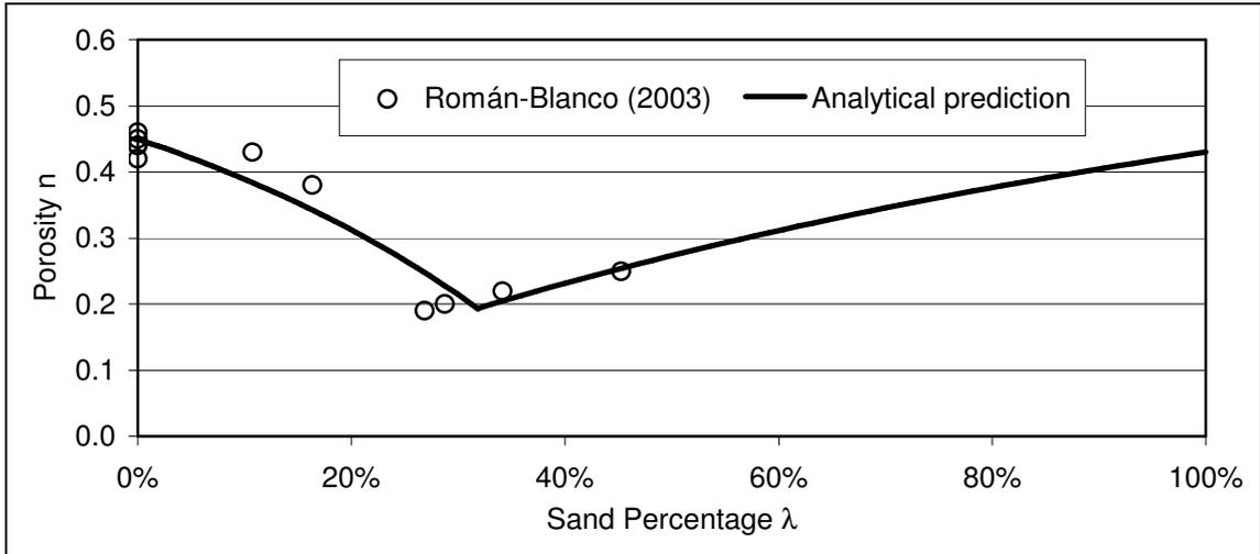
**Figure 3.3 Comparison between analytical prediction and measured porosity of Román-Blanco (2003)**
