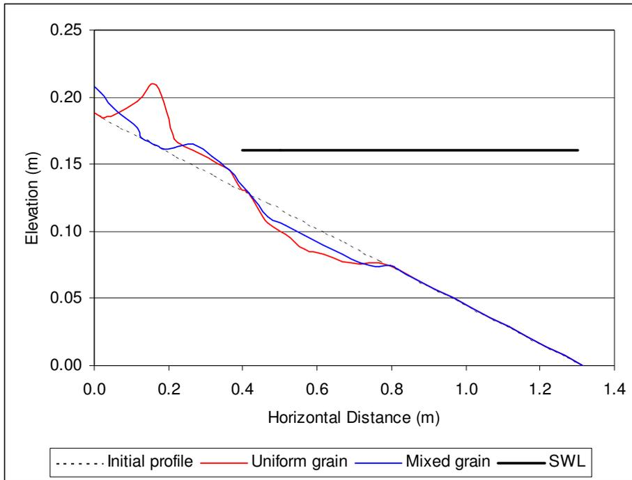
**Figure 4.9 Comparison of gravel (uniform grain) and mixed beach profiles (Random wave condition K:  $f = 1.05\text{Hz}$ ,  $H_s = 0.033\text{m}$ )**
