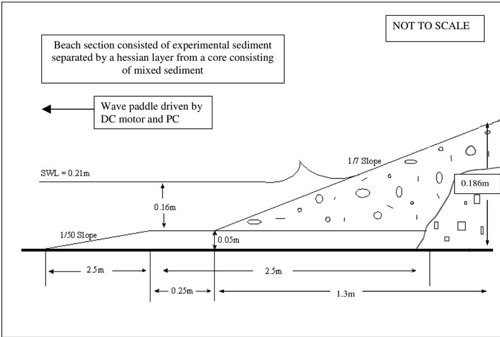
Figure 4.1 Schematic of beach model set-up
