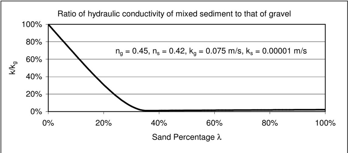
**Figure 3.6 Relative hydraulic conductivity as a function of sand percentage**
