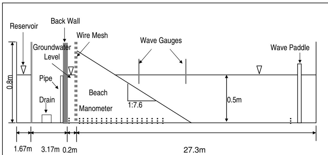
**Figure 5.1 Wave flume, beach layout and instrumentation**
