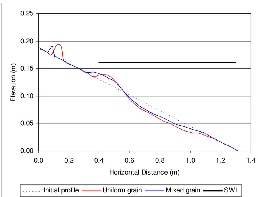
**Figure 4.10 Comparison of gravel (uniform grain) and mixed beach profiles (Random wave condition L:  $f = 1.05\text{Hz}$ ,  $H_s = 0.053\text{m}$ )**
