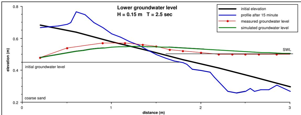
**Figure 5.8 Measured versus modelled groundwater levels for swell conditions ( $T=2.5\text{s}$ ,  $H=0.15\text{m}$ ) on the coarse sand beach, inland groundwater level below SWL**
