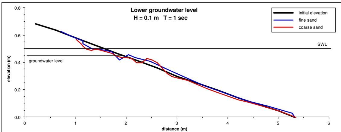
**Figure 5.5 Comparison of fine and coarse sand profiles for storm conditions ( $T=1s$ ,  $H=0.1m$ ), inland groundwater level below SWL**
