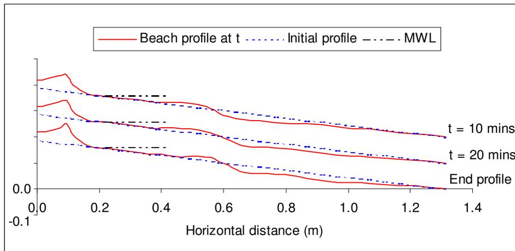
**Figure 4.4 Profiles recorded under random wave conditions (Condition I:  $f=0.53\text{Hz}$ ,  $H_s=0.052\text{m}$ ) with a mixed beach model**
