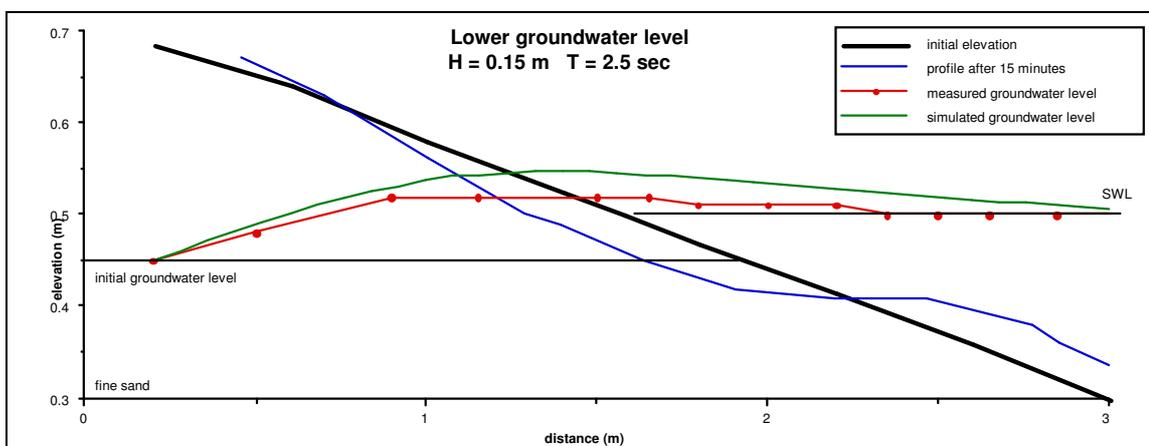
**Figure 5.9 Measured versus modelled groundwater levels for swell conditions ( $T=2.5\text{s}$ ,  $H=0.15\text{m}$ ) on the fine sand beach, inland groundwater level below SWL**
