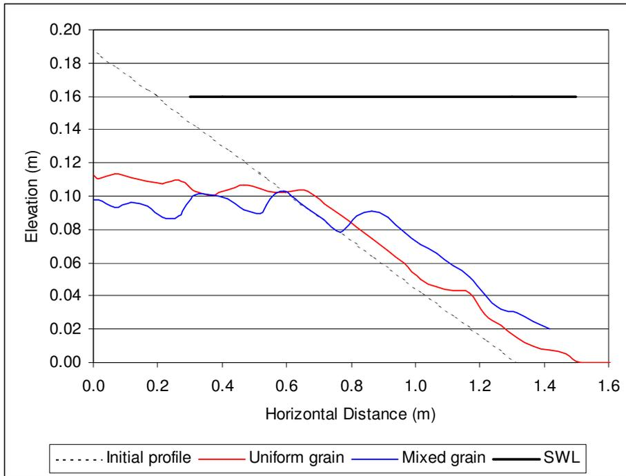
**Figure 4.13 Comparison of gravel (uniform grain) and mixed beach profiles (Monochromatic wave condition H:  $f=1.58\text{Hz}$ ,  $H_s=0.06\text{m}$ )**
