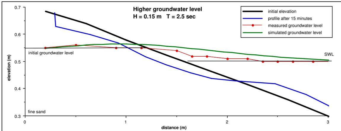
**Figure 5.13 Measured versus modelled groundwater levels for swell conditions ( $T=2.5s$ ,  $H=0.15m$ ) on the fine sand beach, inland groundwater level below SWL**
