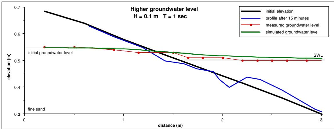
**Figure 5.19 Measured versus modelled groundwater levels for storm conditions (T=1s, H=0.1m) on the fine sand beach, inland groundwater level below SWL**
