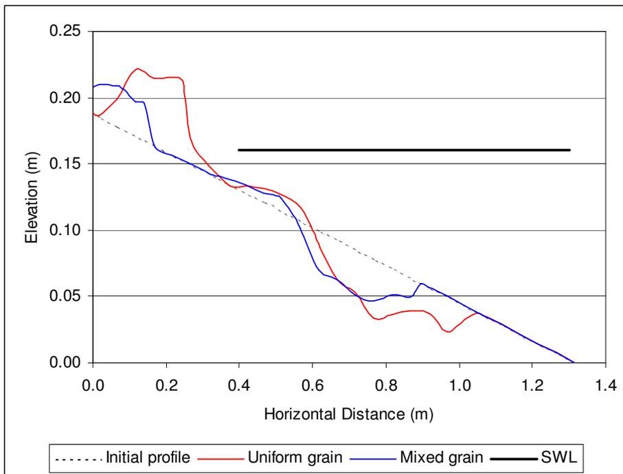
**Figure 4.6 Comparison of gravel (uniform grain) and mixed beach profiles (Monochromatic wave condition B:  $f=0.53\text{Hz}$ ,  $H_s=0.04\text{m}$ )**
