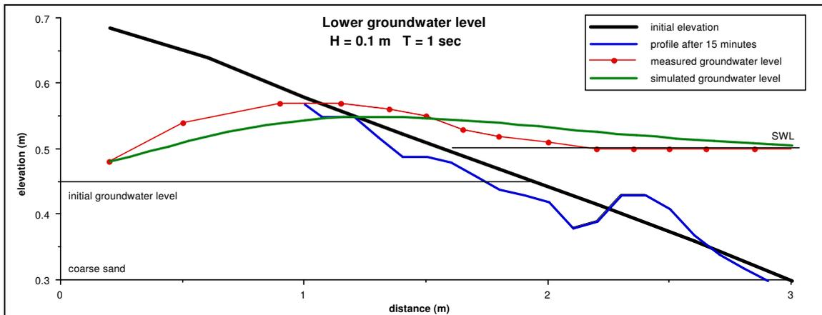
**Figure 5.14 Measured versus modelled groundwater levels for storm conditions ( $T=1s$ ,  $H=0.1m$ ) on the coarse sand beach, inland groundwater level below SWL**
