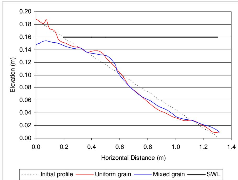
**Figure 4.16 Comparison of gravel (uniform grain) and mixed beach profiles (Random wave condition M:  $f=1.05\text{Hz}$ ,  $H_s=0.069\text{m}$ )**
