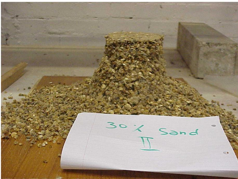
**Figure 3.8 Collapsed “sand castle” ( $\lambda=30\%$ )**
