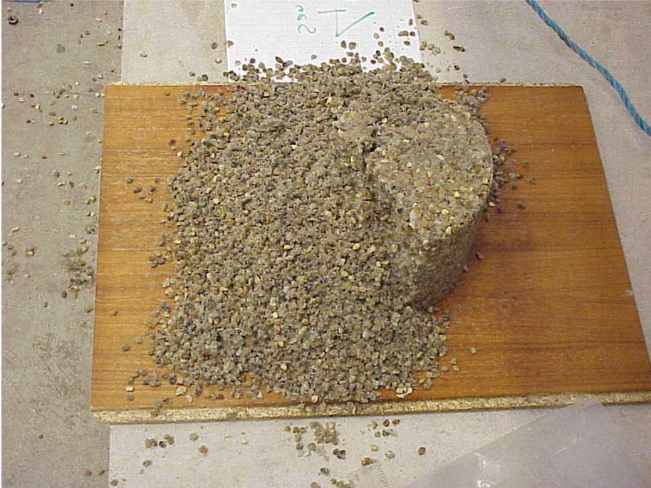
**Figure 3.11 Collapsed “sand castle” ( $\lambda=40\%$ )**
