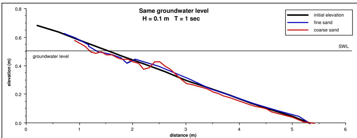
**Figure 5.6 Comparison of fine and coarse sand profiles for storm conditions ( $T=1s$ ,  $H=0.1m$ ), inland groundwater level the same as SWL**
