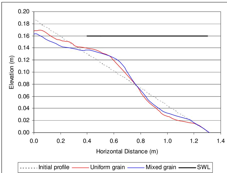
**Figure 4.14 Comparison of gravel (uniform grain) and mixed beach profiles (Random wave condition J:  $f=0.53\text{Hz}$ ,  $H_s=0.084\text{m}$ )**
