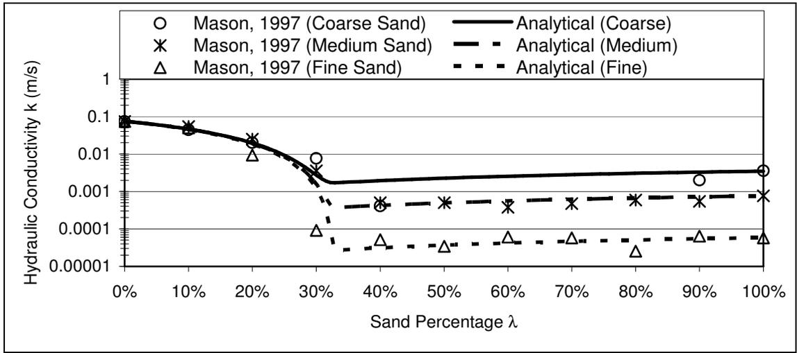
**Figure 3.5 Comparison between analytical prediction and measured permeability of Mason (1997)**
