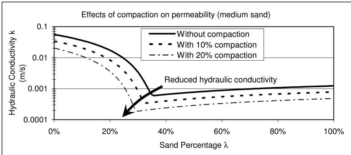
**Figure 3.15 Effects of compaction on hydraulic conductivity**
