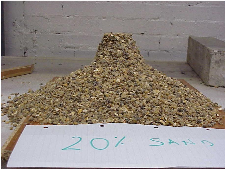
**Figure 3.7 Collapsed “sand castle” ( $\lambda=20\%$ )**
