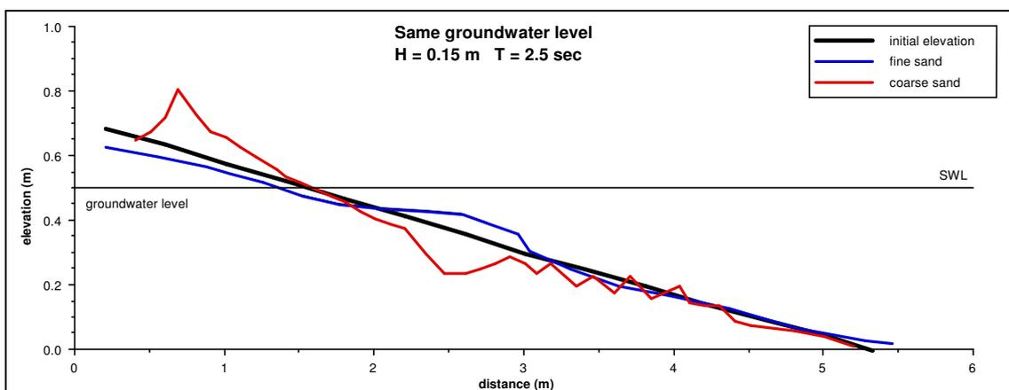
**Figure 5.3 Comparison of fine and coarse sand profiles for swell conditions ( $T=2.5s$ ,  $H=0.15m$ ), inland groundwater level the same as SWL**
