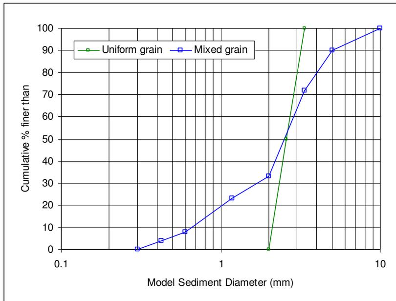
**Figure 4.2 Sediment characteristics of beach models**
