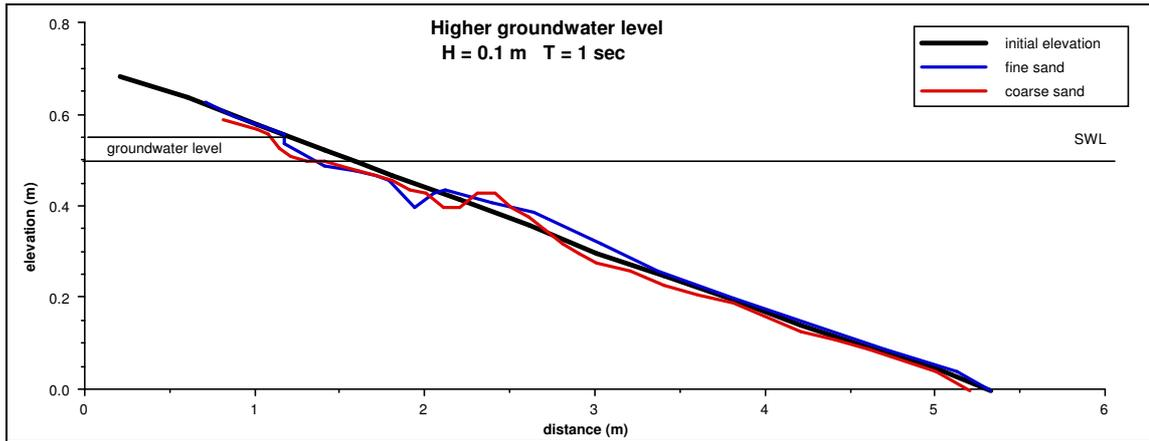
**Figure 5.7. Comparison of fine and coarse sand profiles for storm conditions ( $T=1\text{s}$ ,  $H=0.1\text{m}$ ), inland groundwater level above SWL**
