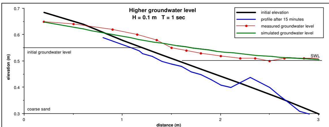
**Figure 5.18 Measured versus modelled groundwater levels for storm conditions ( $T=1s$ ,  $H=0.1m$ ) on the coarse sand beach, inland groundwater level below SWL**
