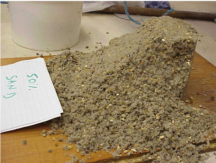
**Figure 3.12 Collapsed “sand castle” ( $\lambda=50\%$ )**
