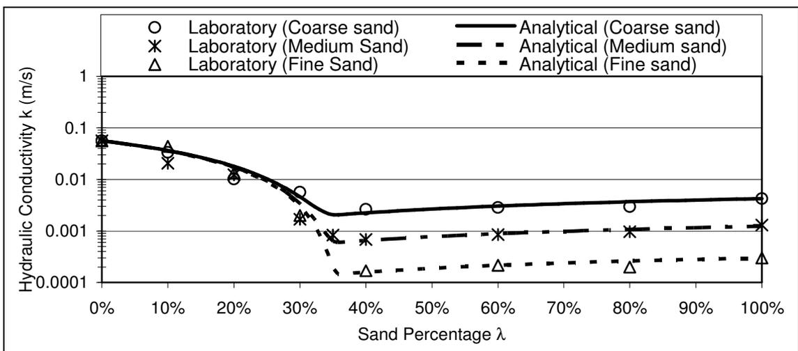
**Figure 3.4 Comparison between analytical prediction and measured permeability (present study)**
