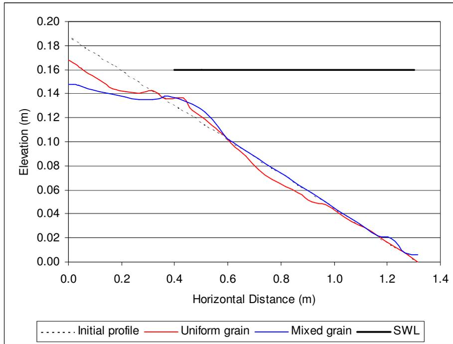
**Figure 4.15 Comparison of gravel (uniform grain) and mixed beach profiles (Random wave condition P:  $f=1.58\text{Hz}$ ,  $H_s=0.052\text{m}$ )**
