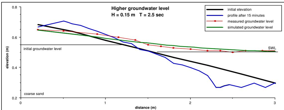
**Figure 5.12 Measured versus modelled groundwater levels for swell conditions ( $T=2.5s$ ,  $H=0.15m$ ) on the coarse sand beach, inland groundwater level below SWL**
