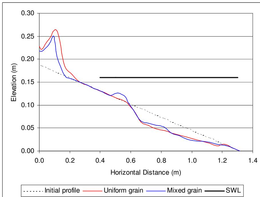
**Figure 4.8 Comparison of gravel (uniform grain) and mixed beach profiles (Random wave condition I:  $f=0.53\text{Hz}$ ,  $H_s=0.052\text{m}$ )**
