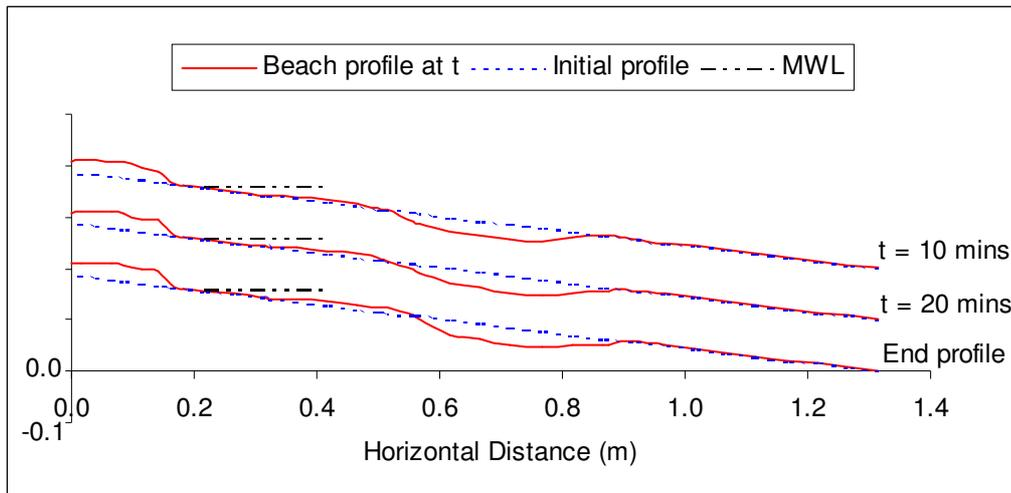
**Figure 4.3 Profiles recorded under monochromatic wave conditions (Condition B:  $f=0.53\text{Hz}$ ,  $H_s=0.04\text{m}$ ) with a mixed beach model**
