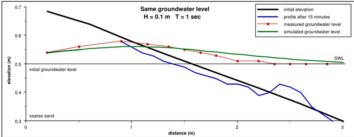
**Figure 5.16 Measured versus modelled groundwater levels for storm conditions ( $T=1s$ ,  $H=0.1m$ ) on the coarse sand beach, inland groundwater level the same as SWL**
