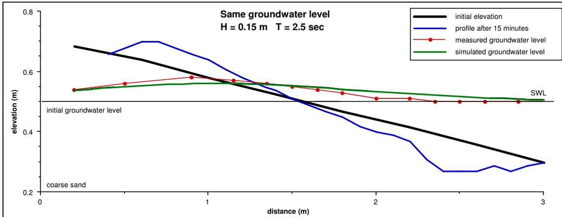
**Figure 5.10 Measured versus modelled groundwater levels for swell conditions ( $T=2.5s$ ,  $H=0.15m$ ) on the coarse sand beach, inland groundwater level the same as SWL**
