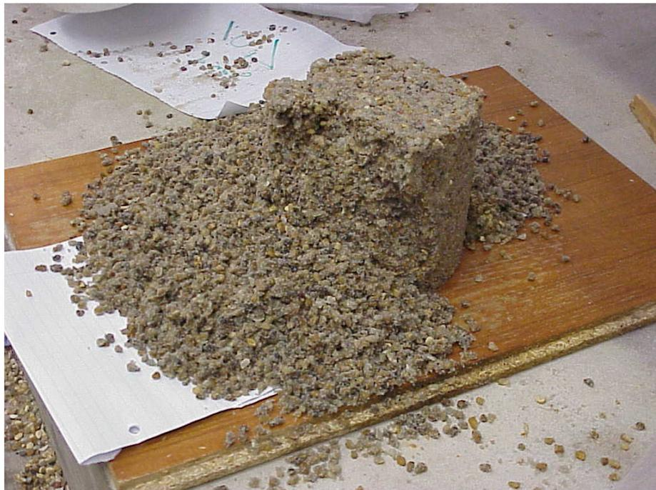
**Figure 3.10** Collapsed “sand castle” ( $\lambda=36\%$ )
