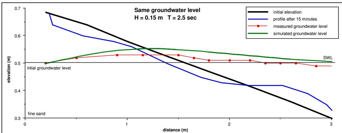
**Figure 5.11 Measured versus modelled groundwater levels for swell conditions ( $T=2.5s$ ,  $H=0.15m$ ) on the fine sand beach, inland groundwater level the same as SWL**
