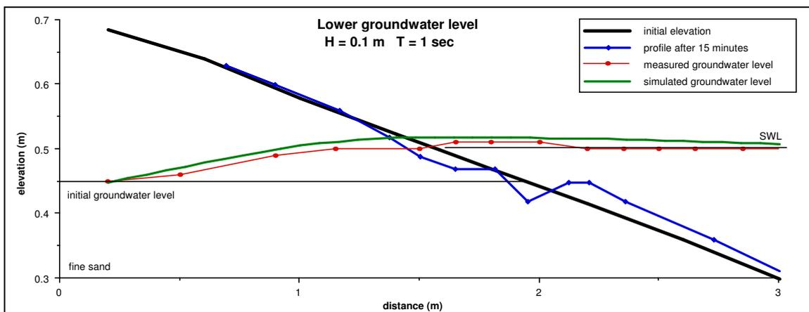
**Figure 5.15 Measured versus modelled groundwater levels for storm conditions ( $T=1s$ ,  $H=0.1m$ ) on the fine sand beach, inland groundwater level below SWL**
