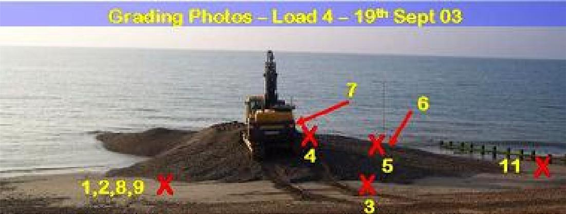
**Figure 6.9 Sediment mound and sample positions**
