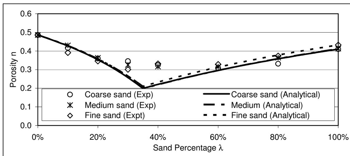
**Figure 3.2 Comparison between analytical prediction and measured porosity (present study)**
