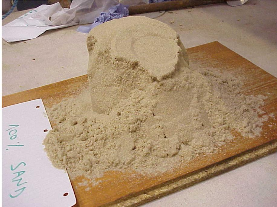
**Figure 3.13 Collapsed “sand castle” ( $\lambda=100\%$ )**
