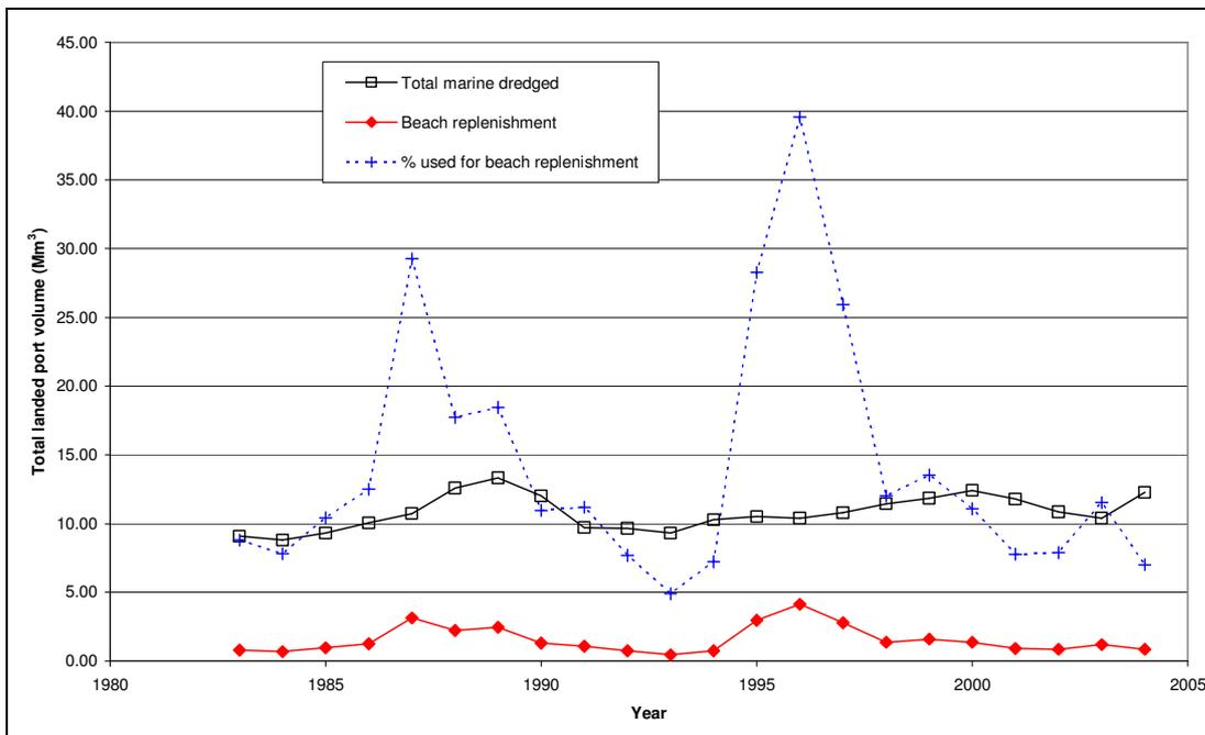
Figure 7.3 Variation in use of dredged sand and gravel for beach replenishment
