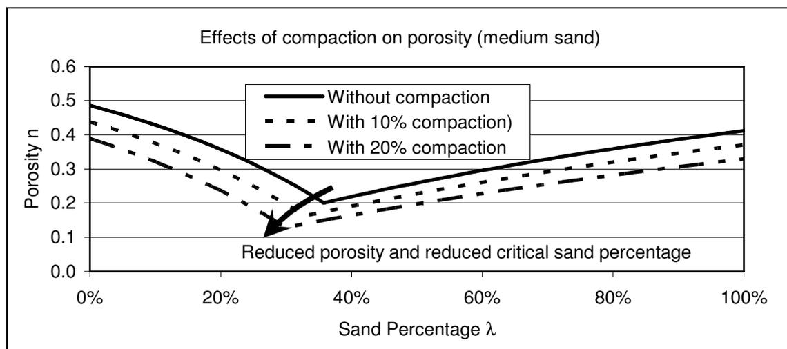
**Figure 3.14 Effects of compaction on porosity**
