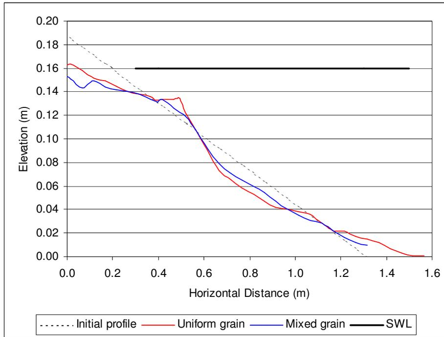
**Figure 4.11 Comparison of gravel (uniform grain) and mixed beach profiles (Random wave condition E:  $f = 1.05\text{Hz}$ ,  $H_s = 0.06\text{m}$ )**
