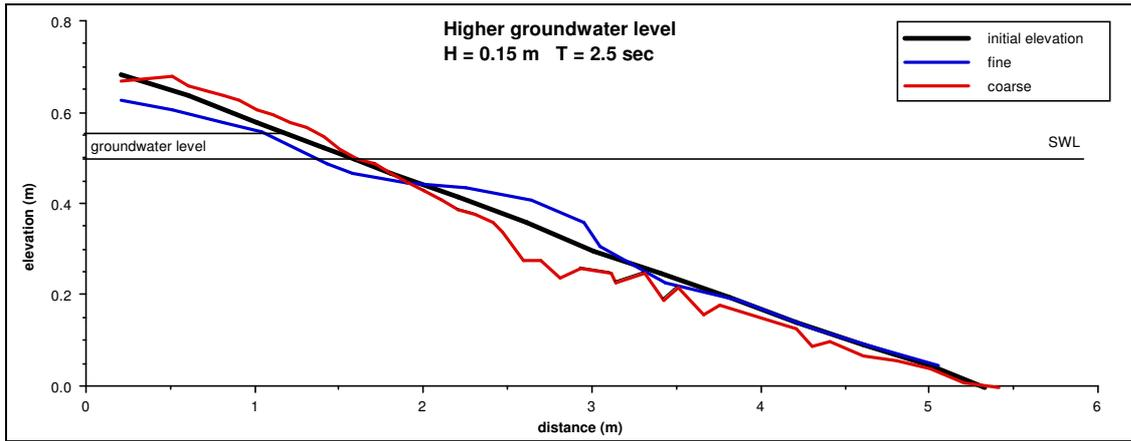
**Figure 5.4 Comparison of fine and coarse sand profiles for swell conditions ( $T=2.5s$ ,  $H=0.15m$ ), inland groundwater level above SWL**
