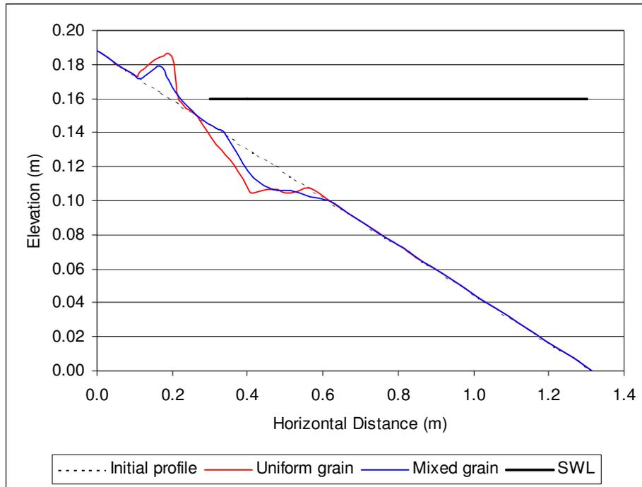
**Figure 4.7 Comparison of gravel (uniform grain) and mixed beach profiles (Monochromatic wave condition C:  $f=1.05\text{Hz}$ ,  $H_s=0.02\text{m}$ )**
