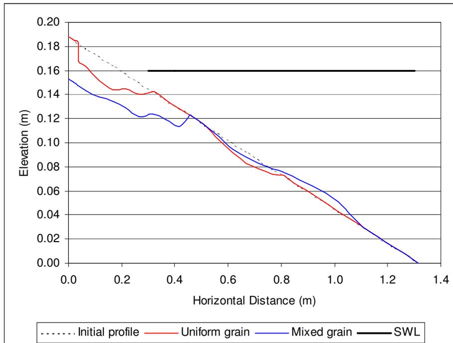
**Figure 4.12 Comparison of gravel (uniform grain) and mixed beach profiles (Monochromatic wave condition G:  $f = 1.58\text{Hz}$ ,  $H_s = 0.04\text{m}$ )**
