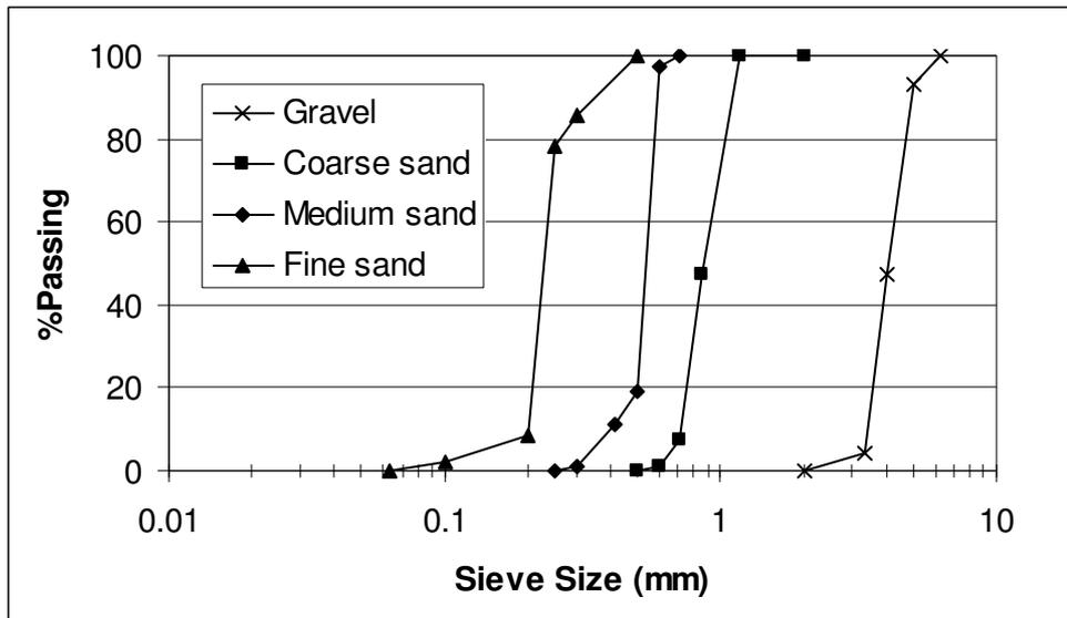
**Figure 3.1 Sediment grading of sand and gravel used for permeability tests**
