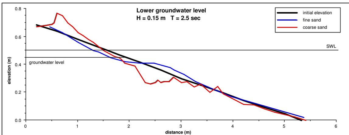
**Figure 5.2 Comparison of fine and coarse sand profiles for swell conditions ( $T=2.5s$ ,  $H=0.15m$ ), inland groundwater level below SWL**
