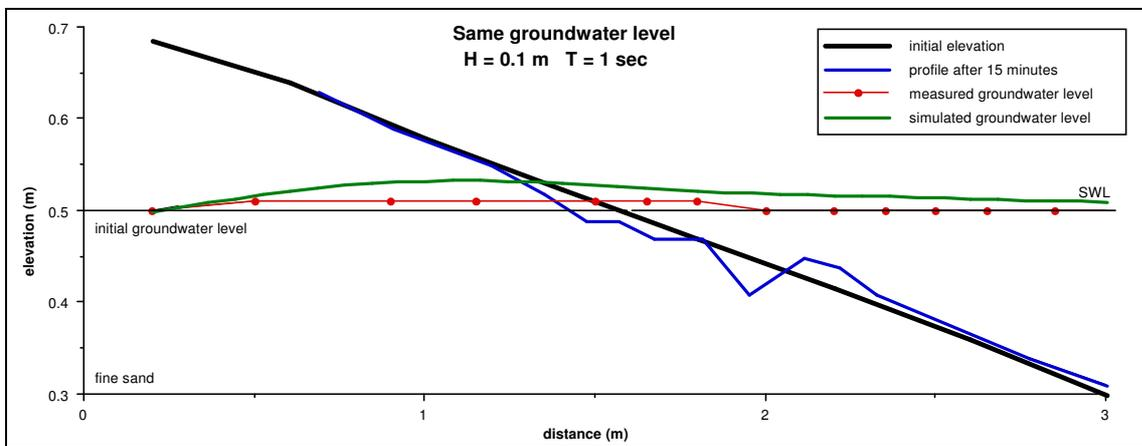
**Figure 5.17 Measured versus modelled groundwater levels for storm conditions ( $T=1s$ ,  $H=0.1m$ ) on the fine sand beach, inland groundwater level the same as SWL**
