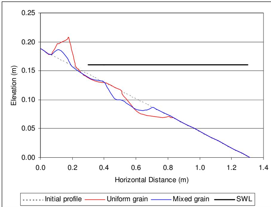
**Figure 4.5 Comparison of gravel (uniform grain) and mixed beach profiles (Monochromatic wave conditions A:  $f=0.53\text{Hz}$ ,  $H_s=0.02\text{m}$ )**
