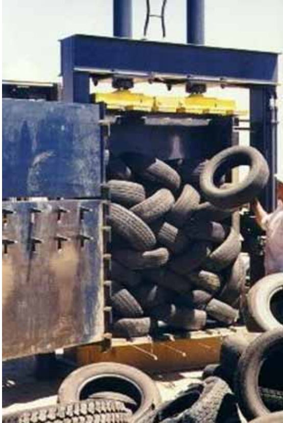
Figure 4.1 Loading baler hopper
