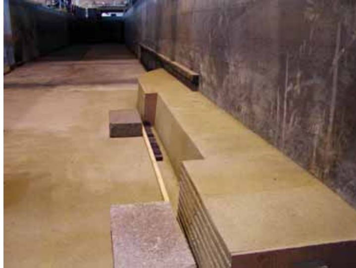
Figure A6.1 Construction of the tyre bale fluvial test section
