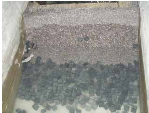
Figure A5.3 Post wave test collapse (Series 2)
