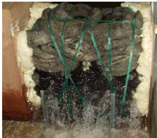
Figure A4.2 Downstream view of small bale test in upright position.
