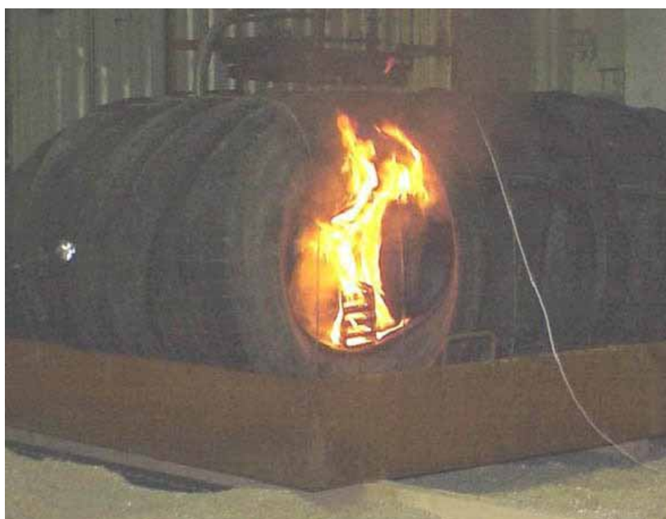
Figure A7.5 Ignition attempt inside the rim of one of the tyres
