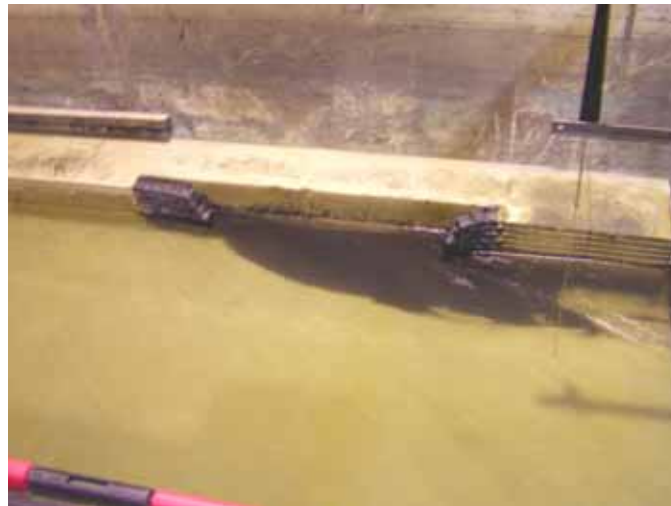
Figure A6.4 Collapse of bank – nominal water depth 0.1m
