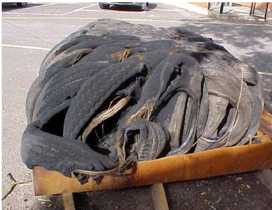
Figure A7.6 Fire damage sustained by the bale
