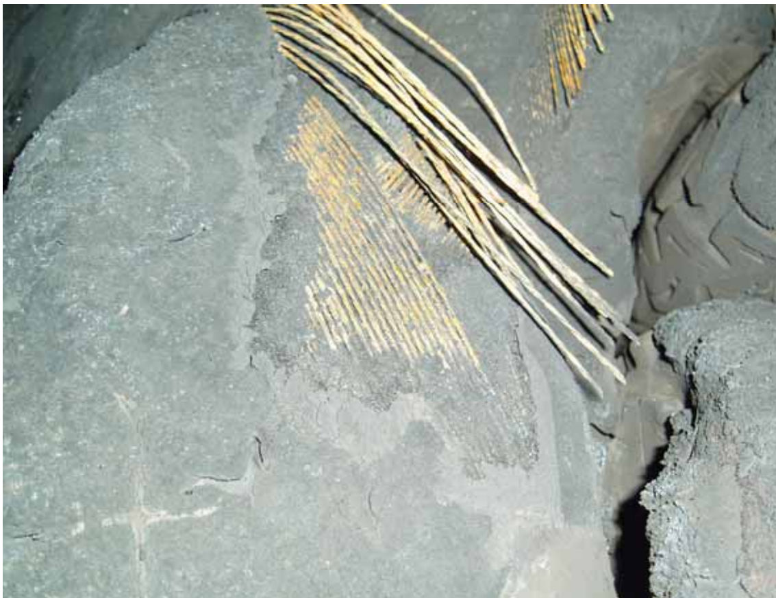
Figure 6.1 Damaged tyre with exposed radial and reinforcing wires
