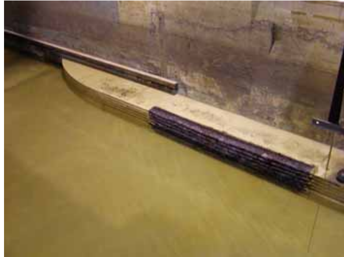
Figure A6.3 Flow conditions during test 3 (mid depth model velocity of 0.335m/s) View from front. Nominal water depth 0.1m
