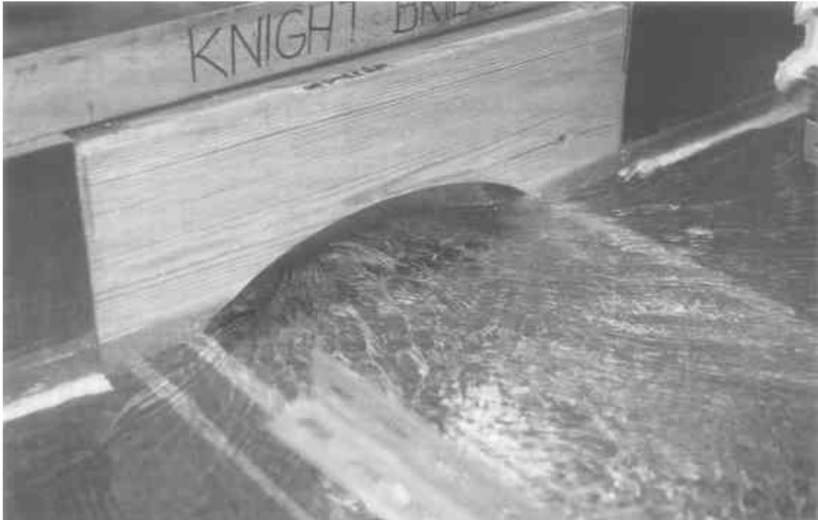
**Figure 10: Observed flow through a model elliptical bridge in a compound channel (Atabay & Knight, 2002).**
