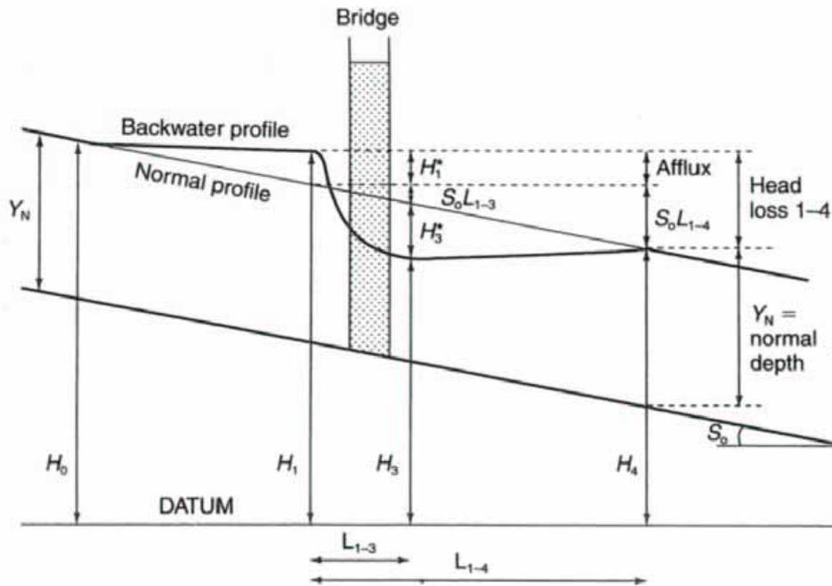
Definition of afflux ( $H_1^* = Y_1 - Y_N$ ) and piezometric head loss for uniform flow at normal depth with the elevation of the water surface measured above a datum. The corresponding water depths at the sections are  $Y_1, Y_2, Y_3$ , etc. Note that the difference in water level between sections 1 and 3,  $\Delta h = H_1^* + S_0 L_{1-3} + H_3^*$ .
