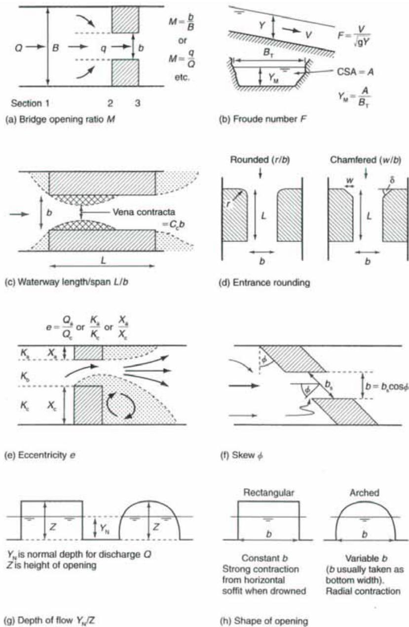
**Figure 1: Summary of principal hydraulic variables affecting the hydraulic performance of a bridge (after Hamill, 1999). (a) Bridge opening ratio,  $M$ ; (b) Froude number,  $F$ ; (c) waterway length/span,  $L/b$ ; (d) entrance rounding; (e) eccentricity,  $e$ ; (f) skew,  $\phi$ ; (g) depth of flow,  $Y_N/Z$ ; (h) shape of opening.**
