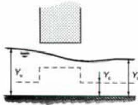
(a) Open channel type flow - channel control
