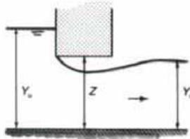
(b) Sluice gate type flow - structure control
