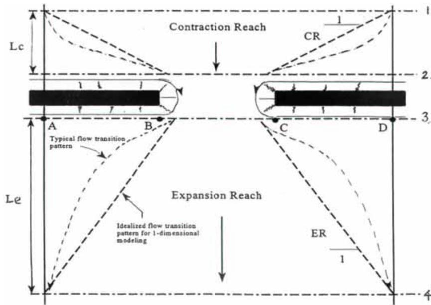
Figure 4: Numbering of cross sections (after HEC-RAS).
