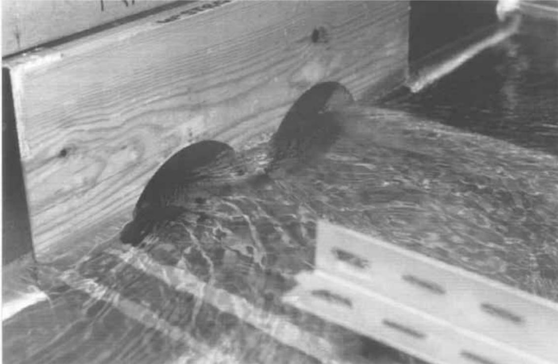
**Figure 11: Observed flow through a model twin arch bridge in a compound channel, viewed from upstream (Atabay & Knight, 2002).**
