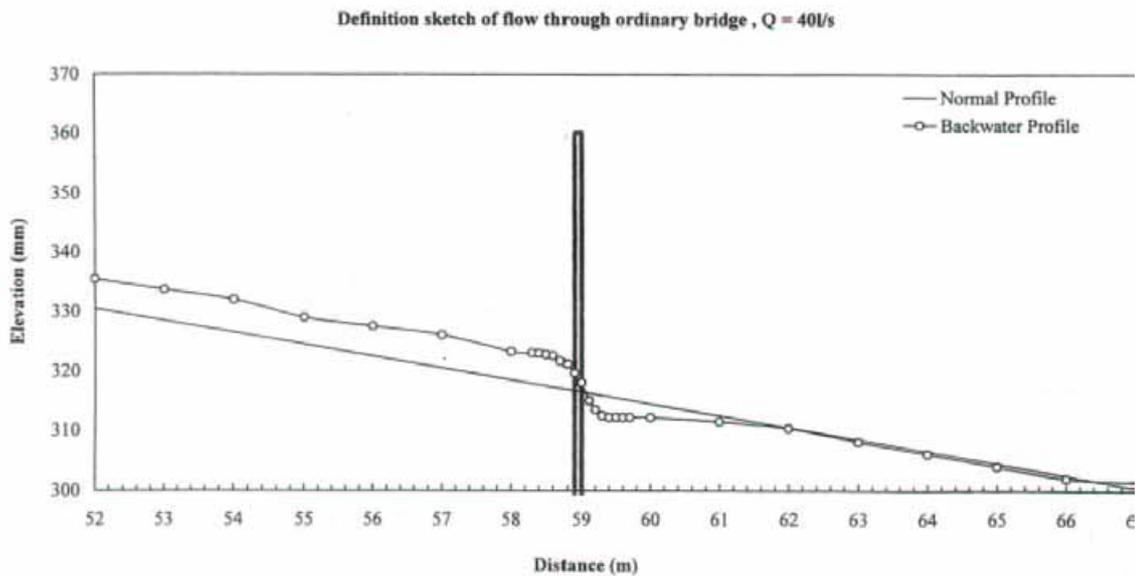
Figure 8: Measured longitudinal water surface profile through a bridge (Atabay & Knight, 2002).
