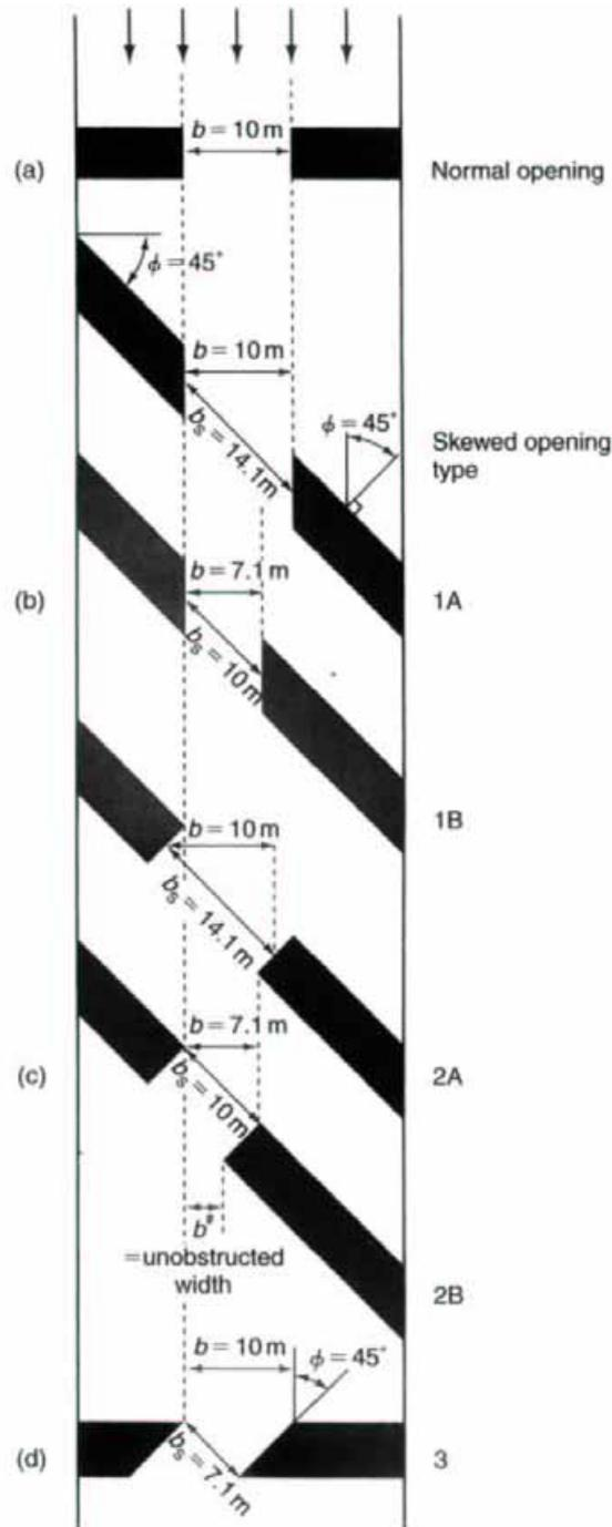
**Figure 2: Comparison of normal and skewed crossings (after Hamill, 1999). (a) Normal crossing; (b) type 1 skew with abutments parallel to the flow; (c) type 2 skew with abutments at  $90^\circ$  to approach embankments; (d) type 3 skew with abutments at an angle  $\phi$  to both the flow and approach embankments.**
