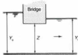
(c) Drowned orifice type flow - structure/channel control
