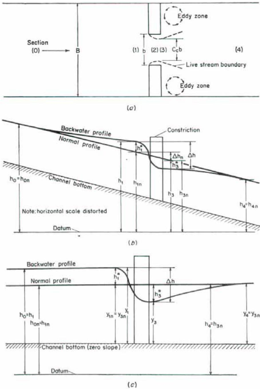
Figure 6: Longitudinal water surface profile through a bridge (after Chow, 1959).
