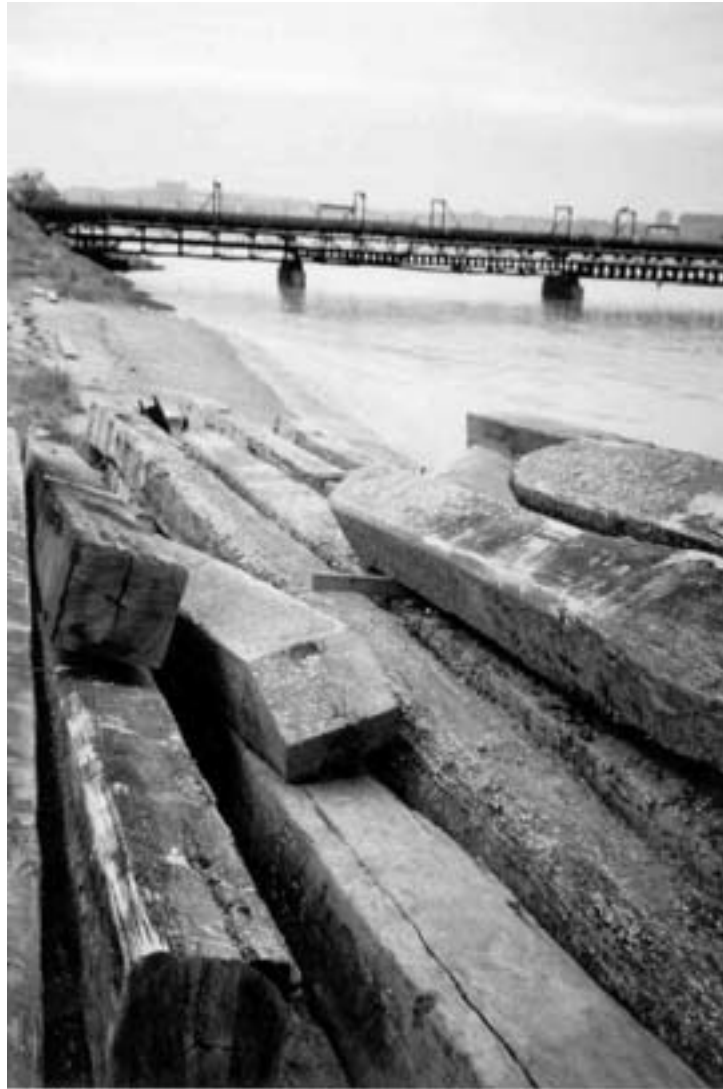
Figure 4.5. Reclaimed hardwood piles awaiting sorting, machining and grading (courtesy John Williams)
