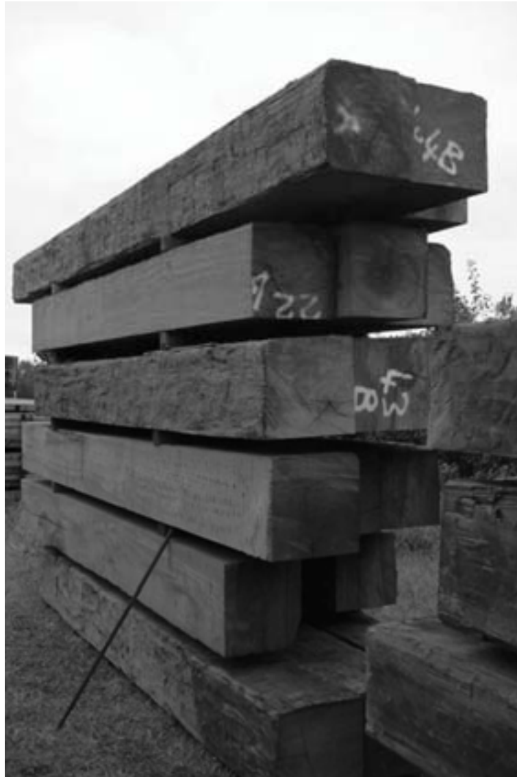
Figure 4.6. Sorted and part machined reclaimed hardwood timber (courtesy John Williams)
