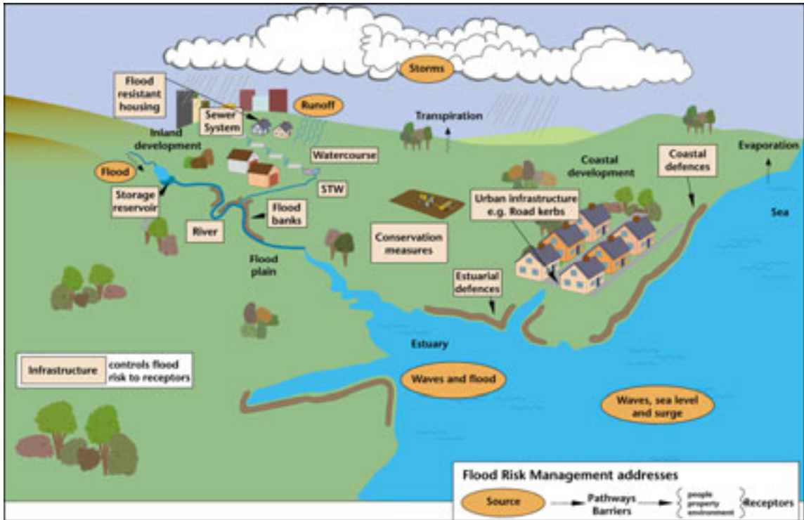
Figure C1.5 Overall flooding system showing sources, pathways and receptors
