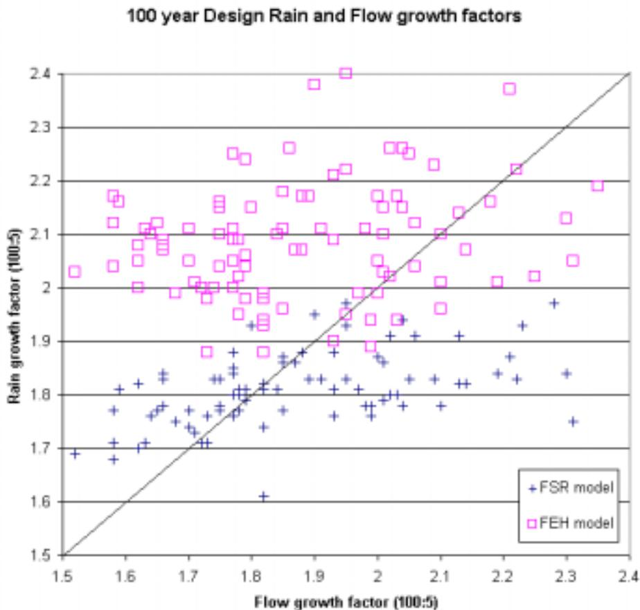
**Figure 6.3 Comparison of steepness of growth curves for FEH and FSR design rainfall and pooled statistical flood frequency analysis.**
