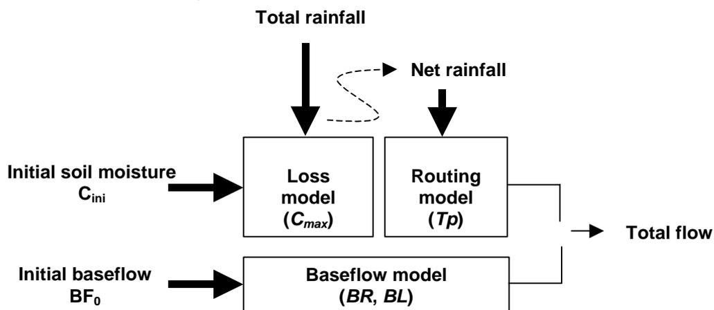
**Figure 3.1 Schematic representation of the ReFH model**
