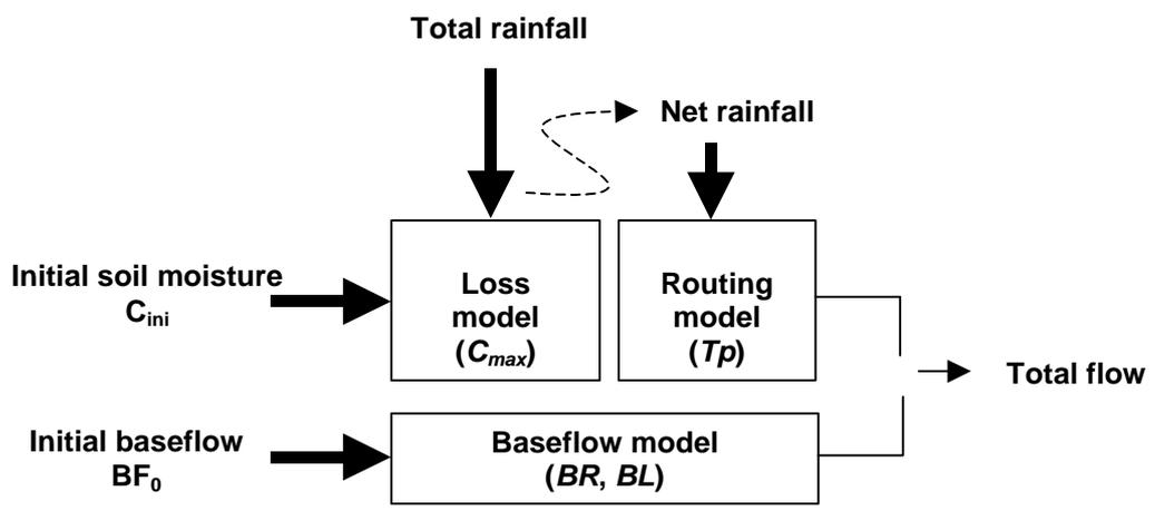
**Figure 6.1 Schematic of the ReFH design model**
