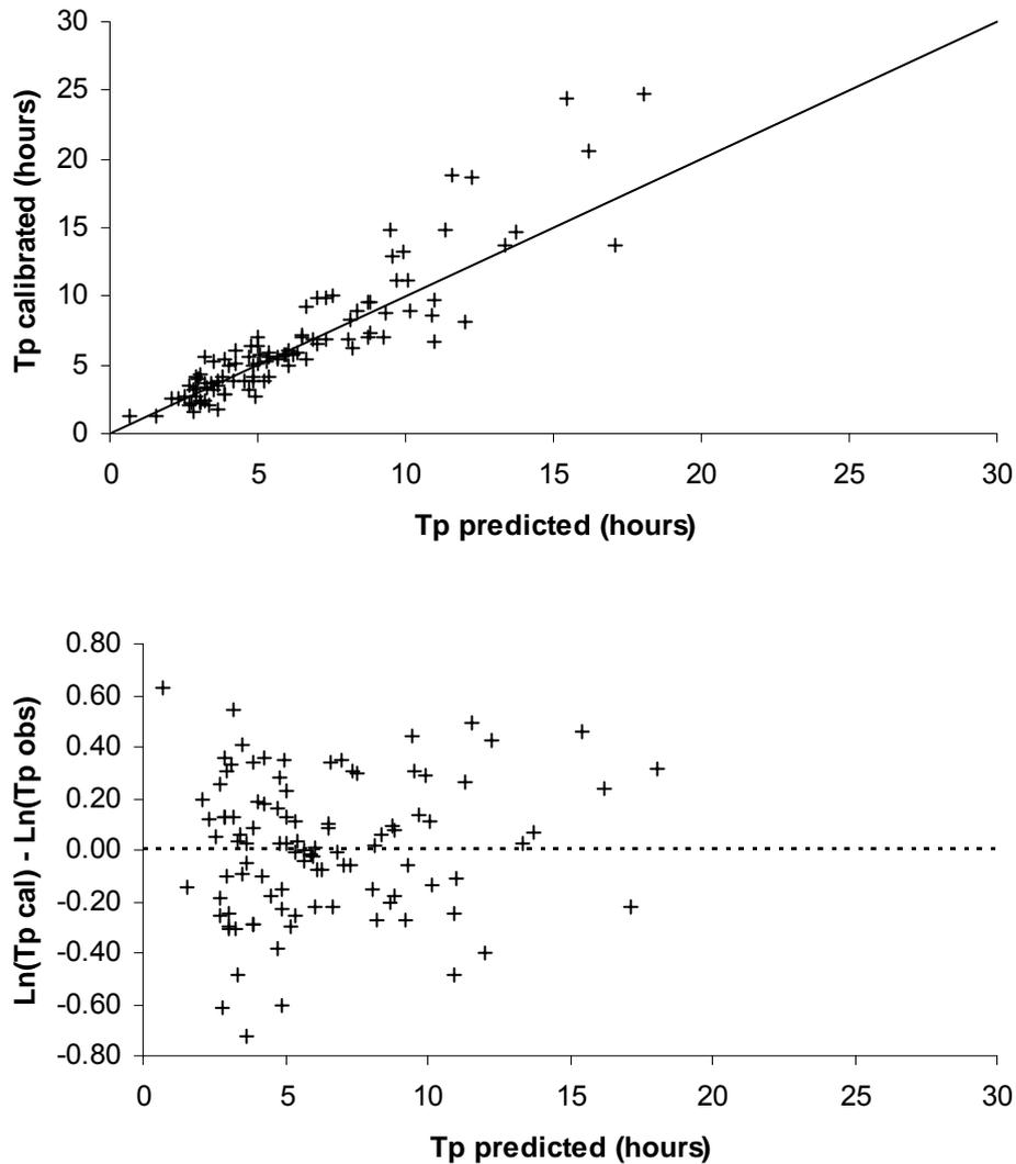
**Figure 7.1 Plot of  $T_p$  observed vs predicted and  $\ln(T_p \text{ predicted})$  against residuals using Eq. (7.4).**
