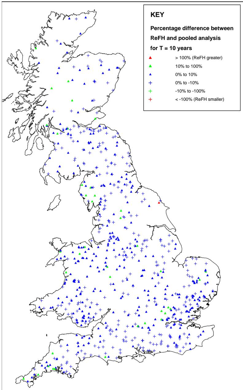
**Figure 8.3 Comparison of the 10 year event estimated using ReFH at an ungauged site compared to the corresponding estimate from pooled statistical analysis at the same gauged site**
