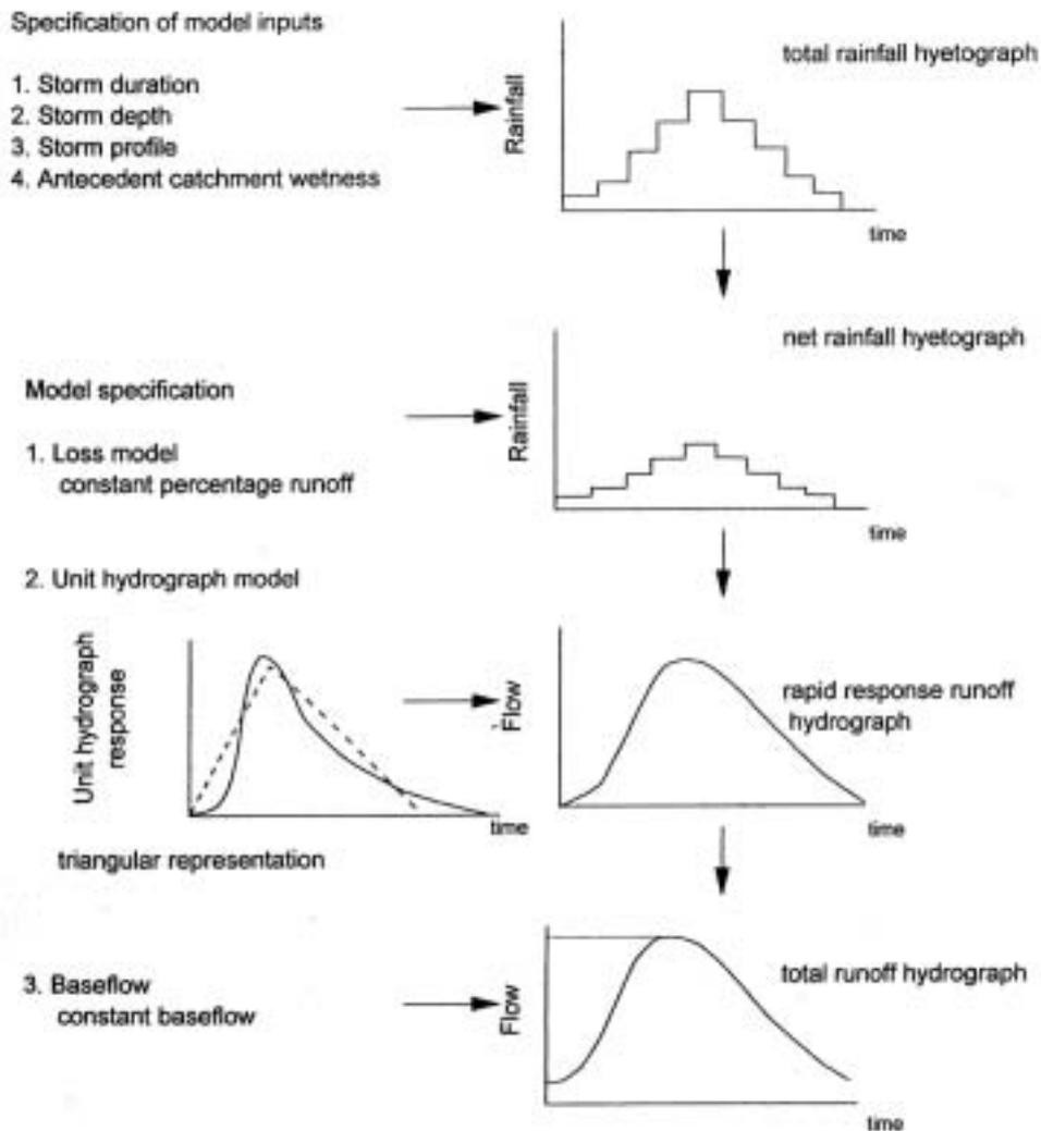
**Figure 1.2** Flood estimation using the FSR rainfall-runoff method (Houghton-Carr, 1999)
