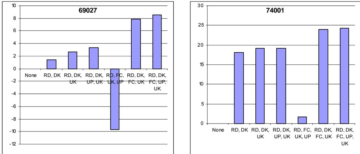
**Figure 4.4 (contd) Sensitivity test showing percentage increase in MSE given a series of fixed parameters**
