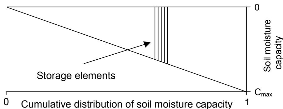
**Figure 3.2 Basin representation of storage elements of different depth**
