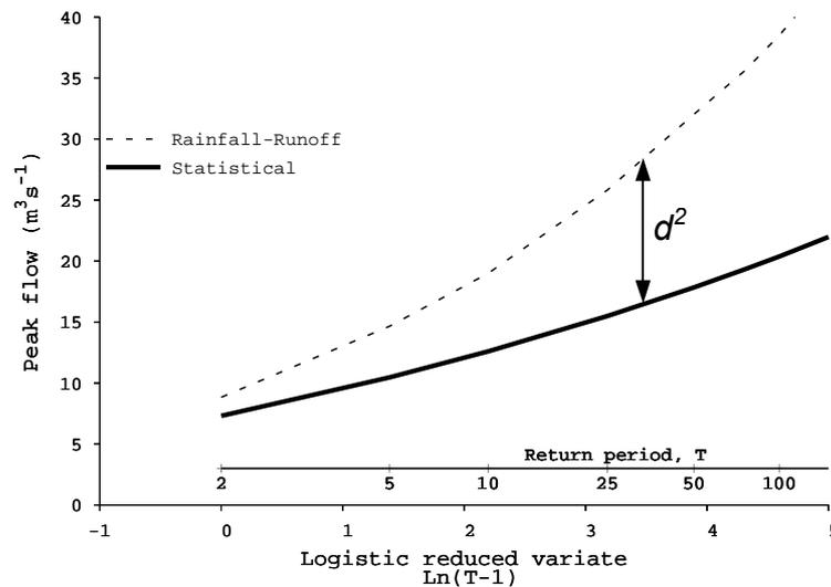
**Figure 6.2** Difference between flood frequency curves from pooled statistical method and as generated by the ReFH model. Calibration performed by minimising  $d^2$  for each return period.
