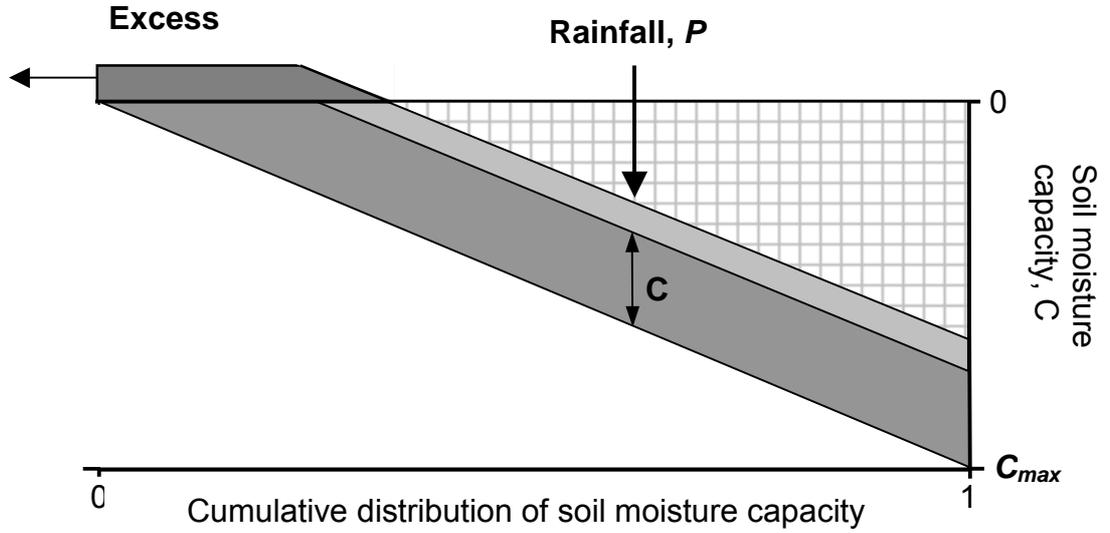
Consequently, the infiltration into a linear PDM can be written as  $i(1-m/SM)^{0.5}$ , where  $i$  is the rainfall intensity. Thus, for the upper zone (moisture content above field capacity), the soil moisture Equation C.1 becomes:
