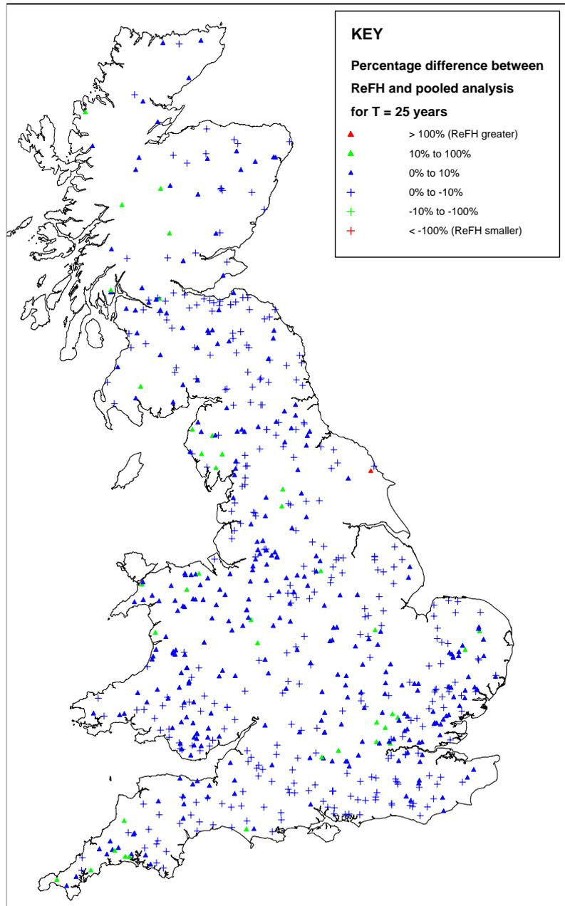
**Figure 8.4 Comparison of the 25 year event estimated using ReFH at an ungauged site compared to the corresponding estimate from pooled statistical analysis at the same gauged site**
