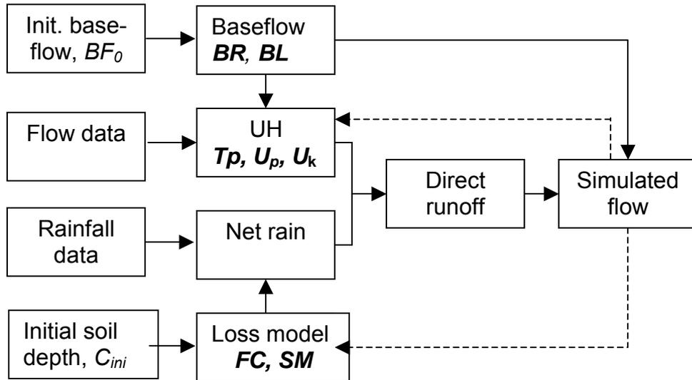
**Figure 4.1 Autocalibration scheme for ReFH**
