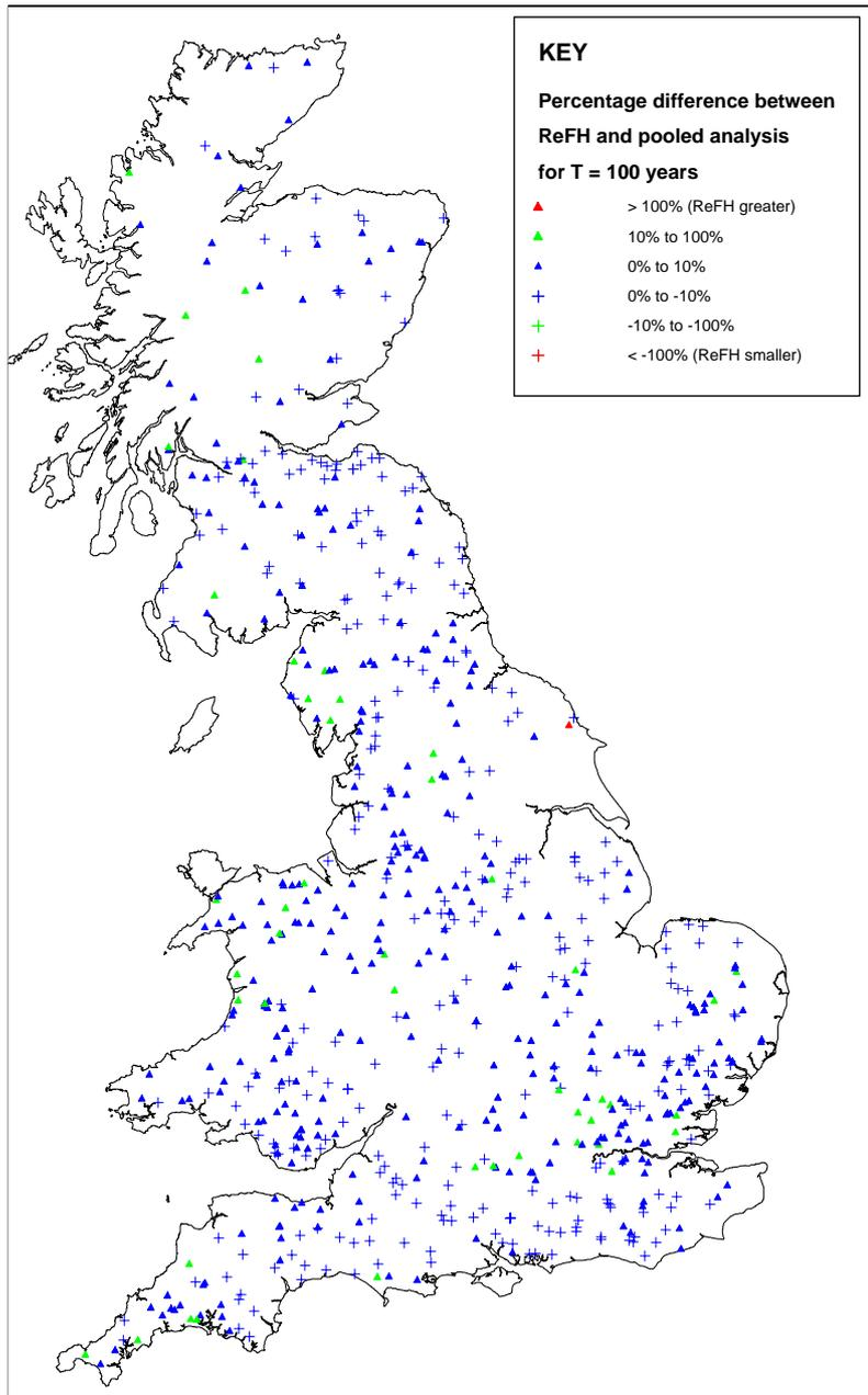
**Figure 8.5 Comparison of the 100 year event estimated using ReFH at an ungauged site compared to the corresponding estimate from pooled statistical analysis at the same gauged site**
