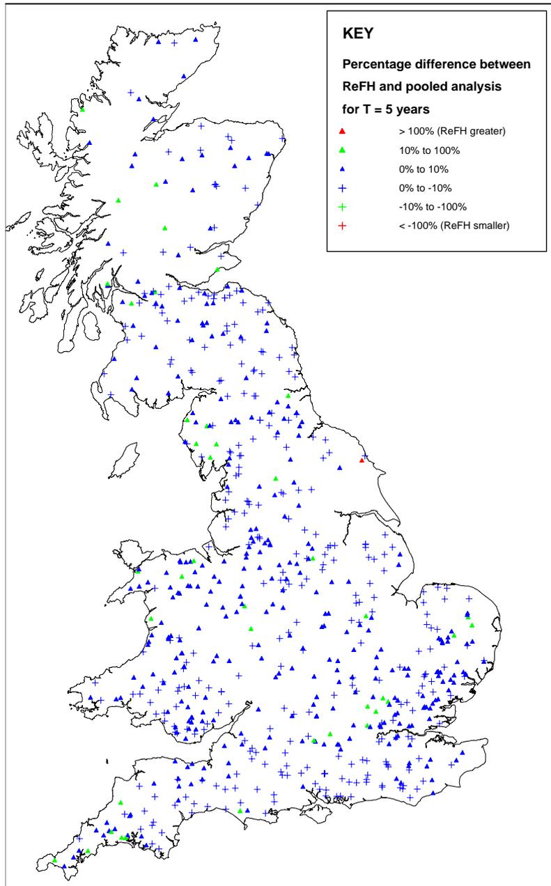
**Figure 8.2 Comparison of the 5 year event estimated using ReFH at an ungauged site compared to the corresponding estimate from pooled statistical analysis at the same gauged site**
