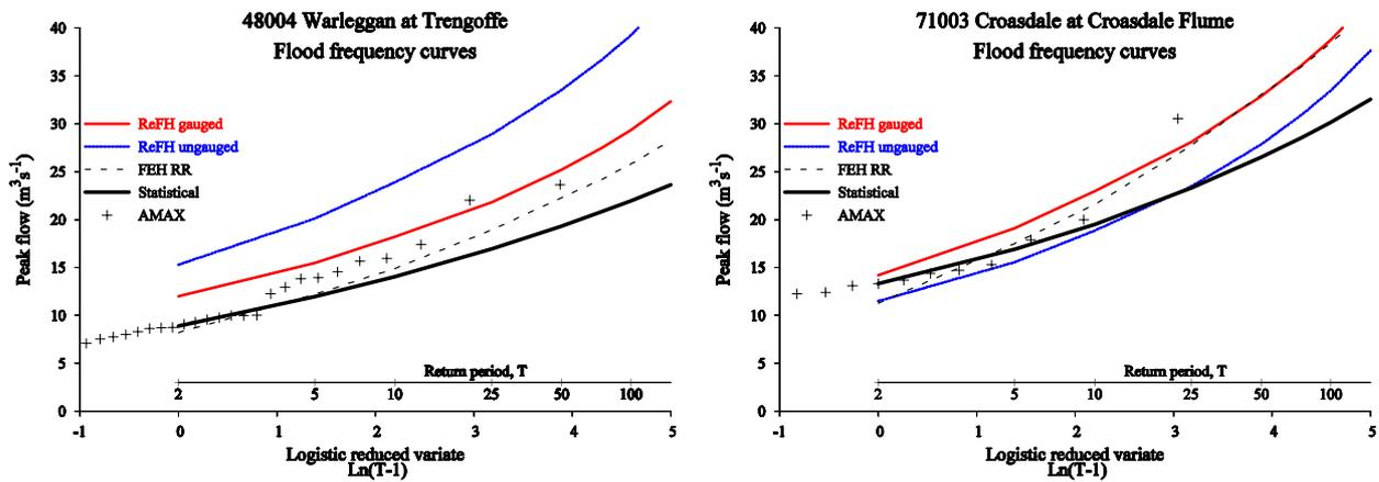
**Figure 8.1 Comparison between FFC derived from observed AMAX series (crosses), ReFH at gauged site (red), ReFH at ungauged site (blue), FEH statistical method (solid black) and the FEH rainfall-runoff method at a gauged site (dashed black)**
