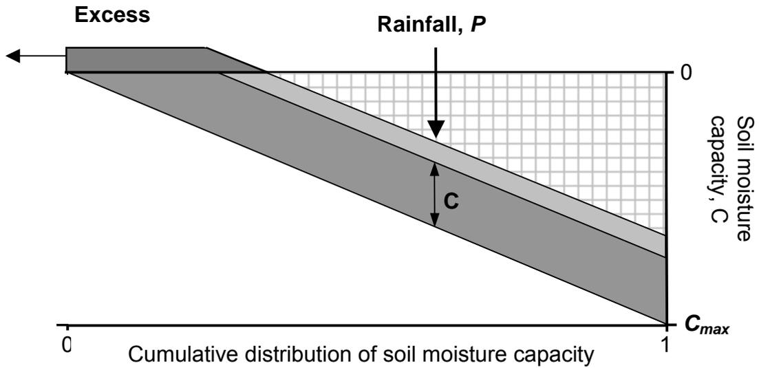
**Figure 3.3 Equal water content,  $C$ , across stores of different capacity**
