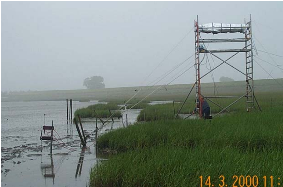
Figure 2.2 Measuring wave attenuation by Spartina vegetation in the Western Scheldt (Mol, 2004)
