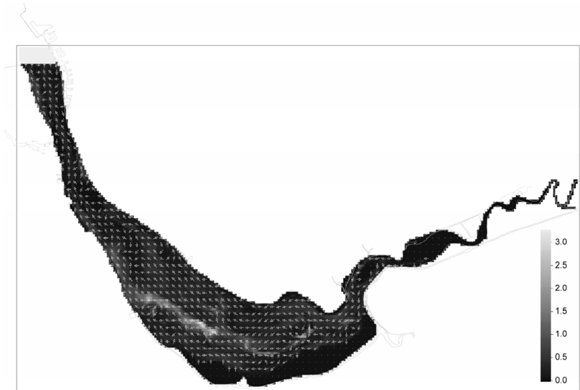
Figure 4.2 Residual currents in the Mersey Estuary near the bed from the high resolution 3-D model (in \text{cm s}^{-1} )
