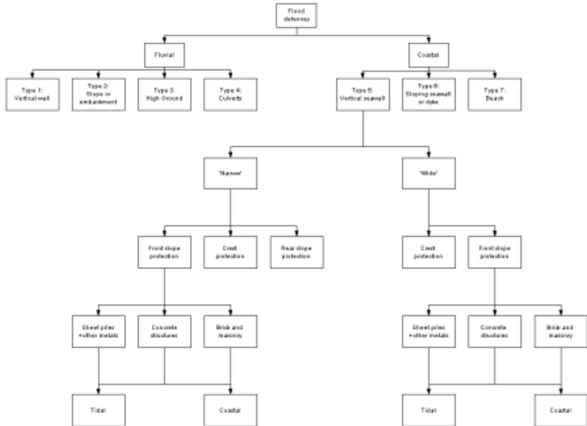
Figure 5.10 Detailed classification of vertical coastal defences
