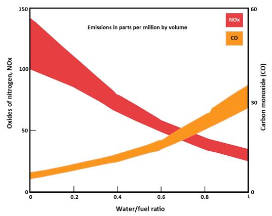
Figure 15 - Emissions of Oxides of Nitrogen (NOx) and Carbon Monoxide (CO)
