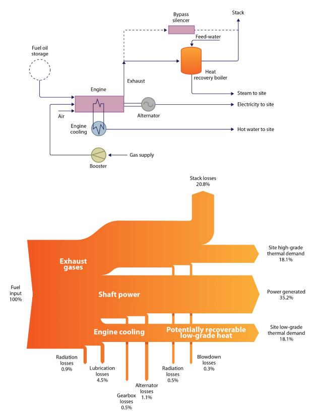
Figure 10: Energy flow diagram for a CHP engine with Heat Recovery Boiler
