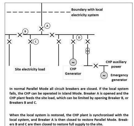
If the failure of the local system trips the CHP generator, it can be restarted using power supplied from the emergency generator to the CHP auxiliary power system.
