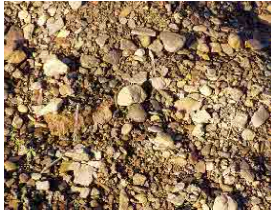
Typical dredged section – no toe left, and predominance of gravel and pebbles in dredgings
