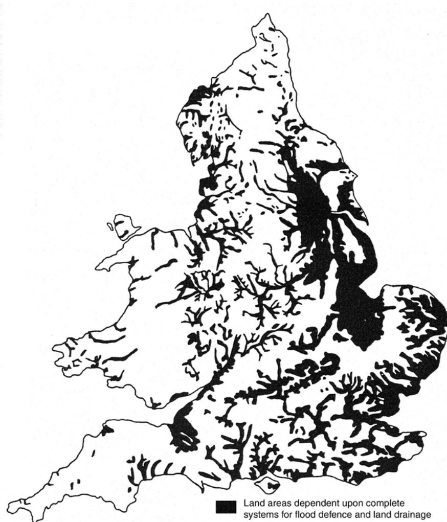
Figure 5.2 Extent to which floodplains are occupied by out-of-bank flows with a 100-year return period.
