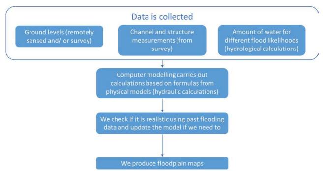
Figure 7. How we model floodplains
