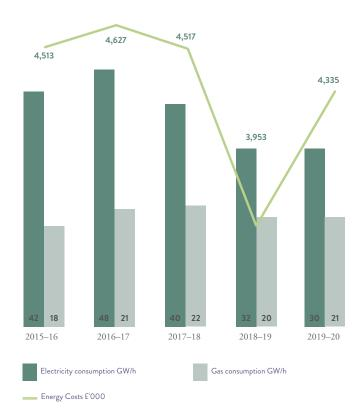
The energy consumption figures include both consumed grid energy and 'on-site' generated energy. The significant change in energy consumption per tonne for the last two years is in part a result of the removal of on-site casting of non-ferrous metals.
