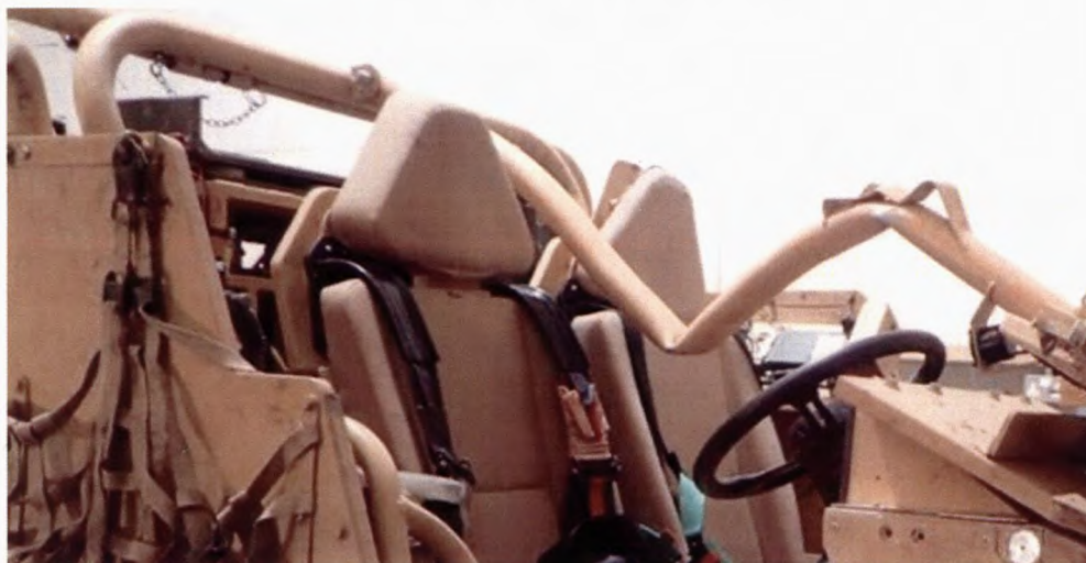
Figure 1.4. 47 – JACKAL [REDACTED] Cutter Bar post-accident
