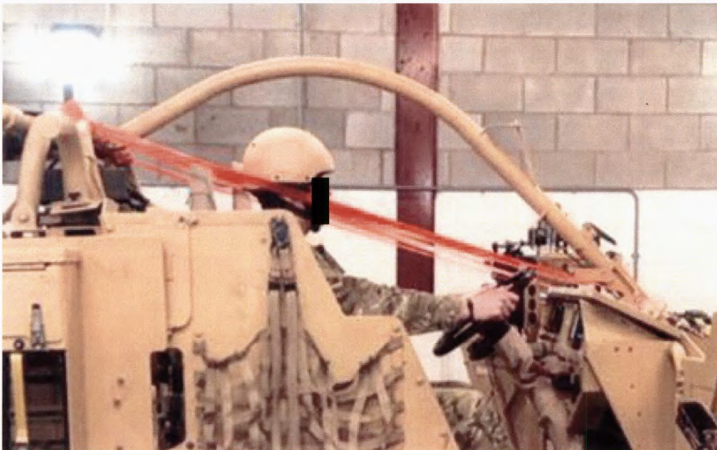
Figure 1.4. 46 – Roll Over Protection System to bulkhead analysis
