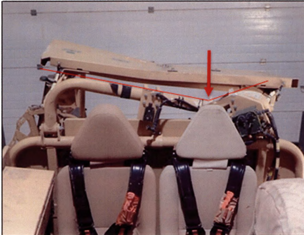
Figure 1.4. 45 – [REDACTED] rear seats and Roll Over Protection System deformation
