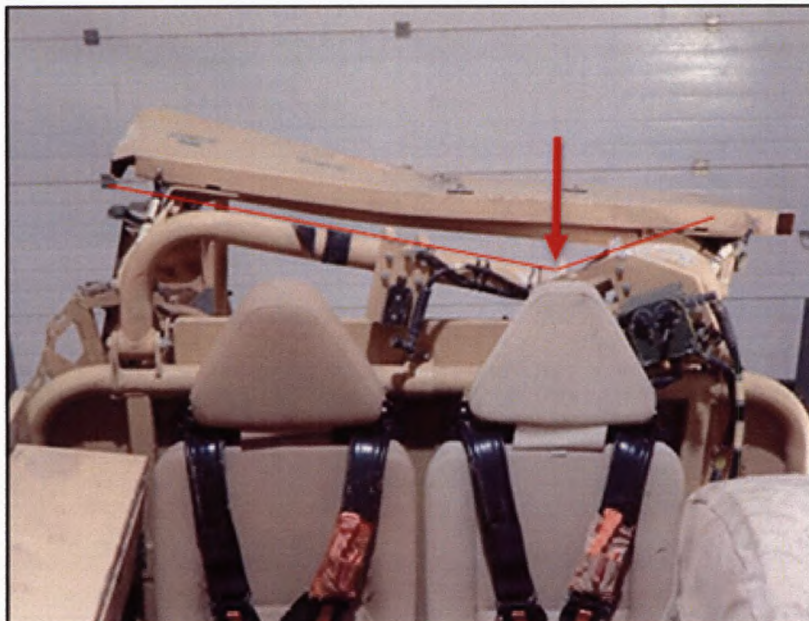
Figure 1.4. 14 – [REDACTED] rear Roll Over Protection System damage
