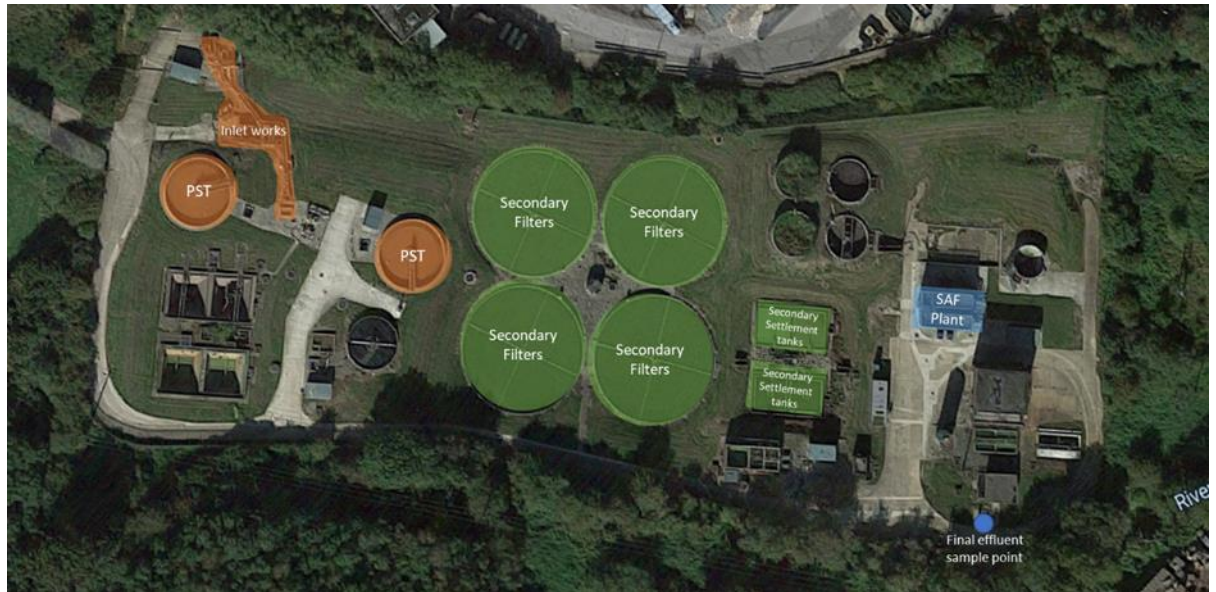
Figure 1: Basic Installation. The orange highlighting represents preliminary processes, the green secondary treatment, and the blue tertiary treatment. "PST" stands for "Primary Settlement Tanks" and "SAF" stands for "Submerged Aerated Filter".
