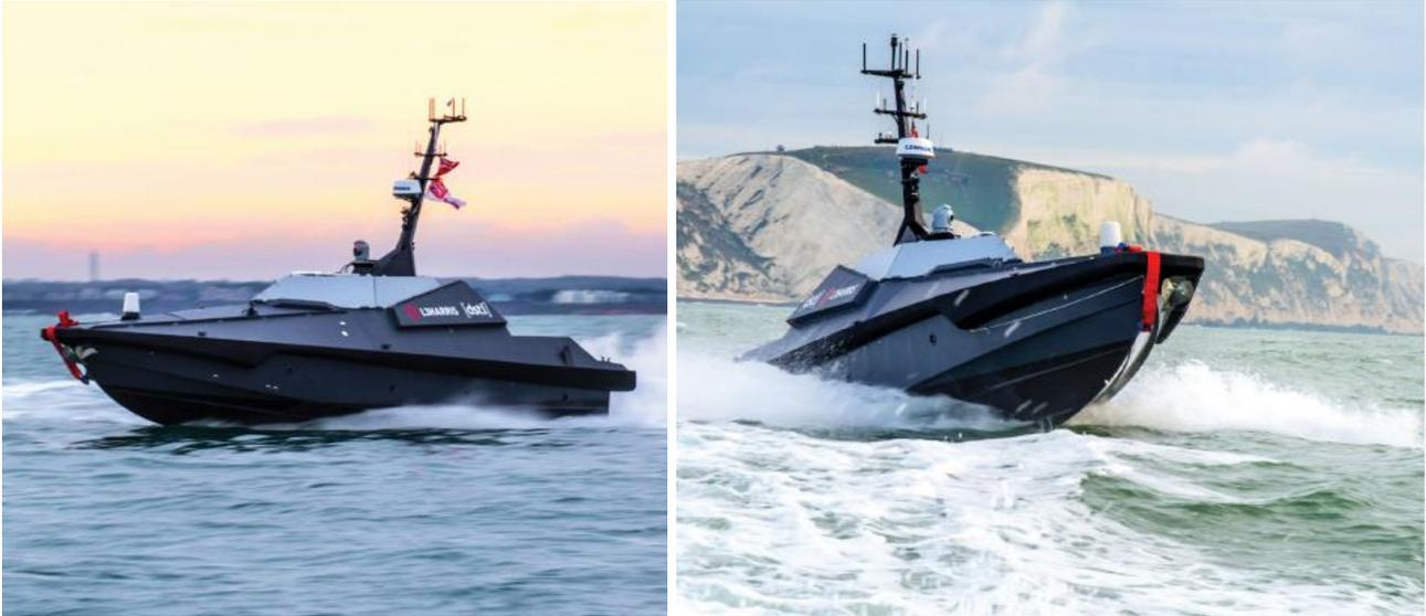
**Dstl, in collaboration with L3Harris has launched a novel Unmanned Surface Vessel (USV) designed to act as a research testbed for exploring higher levels of USV autonomy.**
