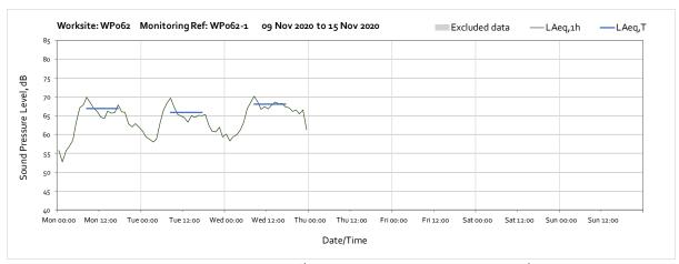
Note: Missing data between 00:00 on Thursday 12<sup>th</sup> November and 13:00 on Tuesday 24<sup>th</sup> November was due to an outage caused by a fault with the monitor due to a blown fuse.
