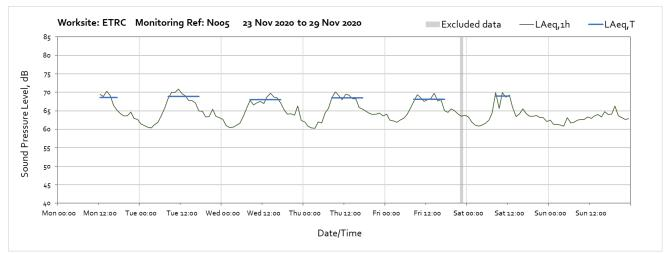
Note: Missing data from 01:00 on Sunday 22<sup>nd</sup> November until 12:00 on Monday 23<sup>rd</sup> November was due to a temporary loss of site power (including power to the monitoring station) which was subsequently restored.
