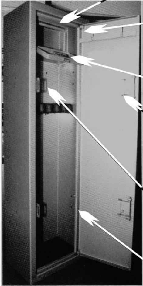
A cabinet is usually made from steel sheet, by continuously welded or bend construction to prevent insertion of bars, chisels etc
