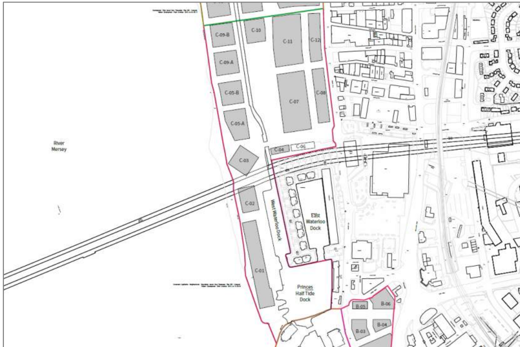
Figure 1.1: Central Docks Development Plots (C-01 to C-12). Image taken from Parameter Plan 005 Liverpool Waters Development Plots. Drg. No. 1868-VW-005 (Planit I.E. Limited, 2018).
