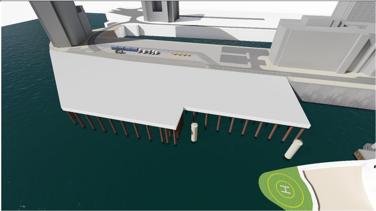
Image 6 – Southern end of the deck completed to allow works on the building to commence (note the deck will never look as open as this as the building frame will have commenced at this stage.
