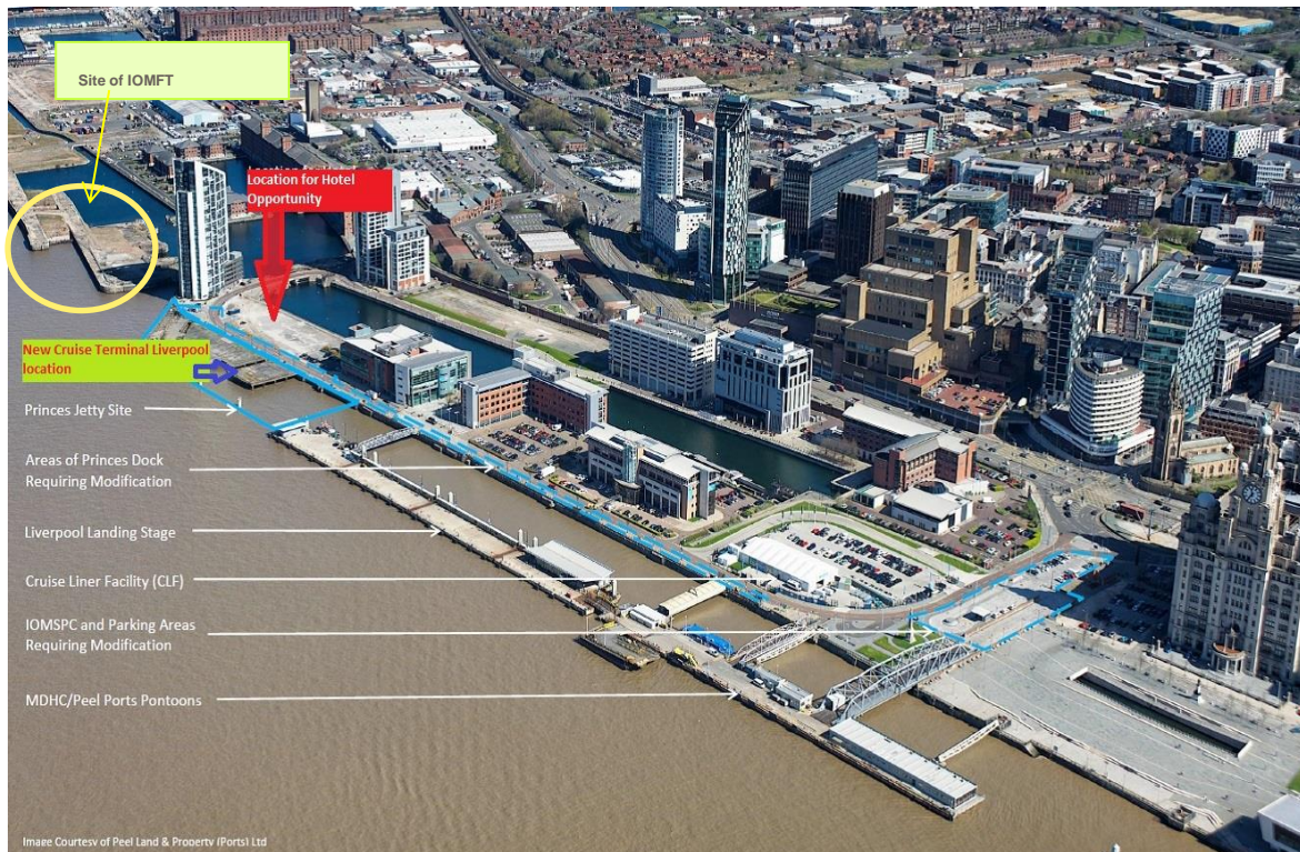
Figure 2: Location Plan: Existing Liverpool cruise landing stage and site of Liverpool cruise Terminal
